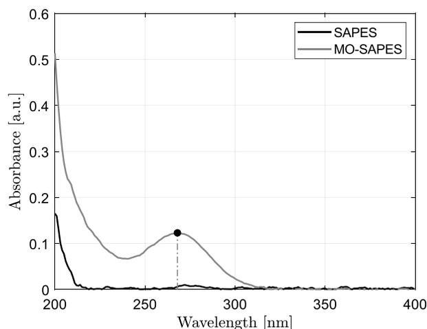
**Fig. 9** UV-vis spectra of SAPES and MO-SAPES
