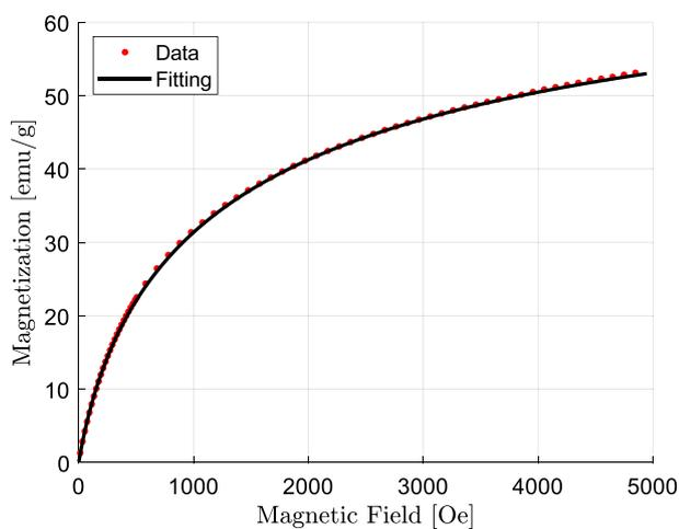
**Fig. 2** Magnetization curve for as-made iron oxide NPs
