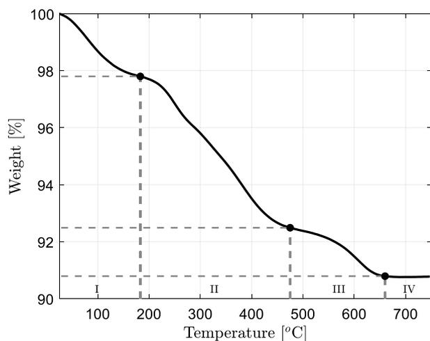
**Fig. 4** TGA thermogram of the SPION sample. Four decomposition stages are identified: (I) water desorption (25–180 °C), (II, III) citrate decomposition in two steps (180–660 °C) and (IV) steady-state (> 660 °C)
