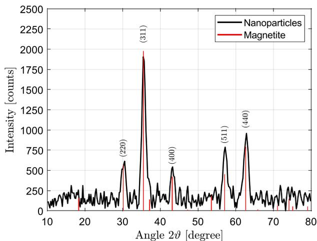
**Fig. 1** XRPD pattern for as-made iron oxide NPs. The main crystal-line planes are indexed with corresponding Miller indices of cubic  $\text{Fe}_3\text{O}_4$ —magnetite (ICDD card no:88-0315; COD card no: 9005837)
