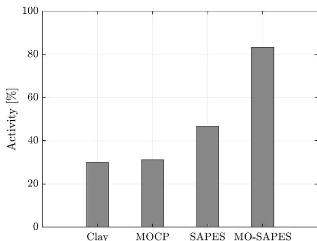
**Fig. 10** Activities for only clay, MOCP, SAPES and MO-SAPES samples for turbidity removal via magnetic separation
