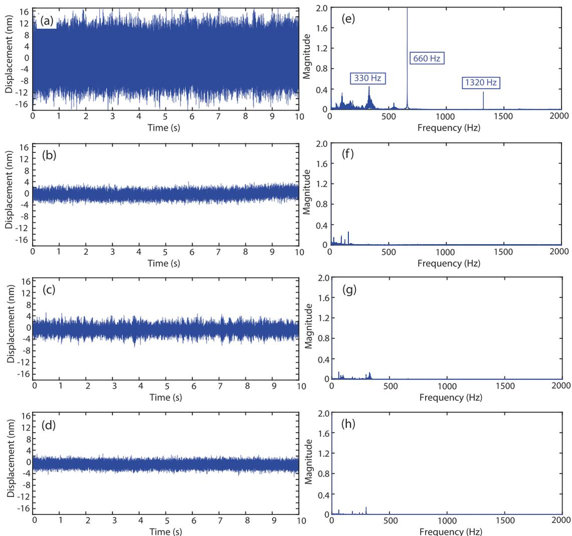
**FIG. 2.** Stability measurements on the dry sample holder. The displacement plots in the time domain are shown in the left column, and the corresponding spectra in the frequency domain are shown to the right. Four separate measurements are presented: With the main turbo pump connected to the microscope chamber and turned on [(a) and (e)] and off [(b) and (f)]. With the main turbo pump decoupled from the microscope chamber and turned on [(c) and (g)] and off [(d) and (h)].
