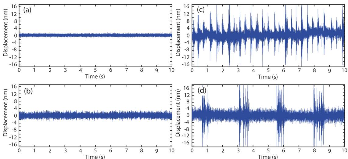
**FIG. 4.** Displacement measurements on the cryo sample holder under four different conditions. (a) Without liquid nitrogen, (b)  $>10$  min after refilling the cryostat and the cryo sample holder with liquid nitrogen, (c) a few moments after refilling the cryo sample holder with liquid nitrogen, and (d) a few moments after filling the cryostat with liquid nitrogen.
