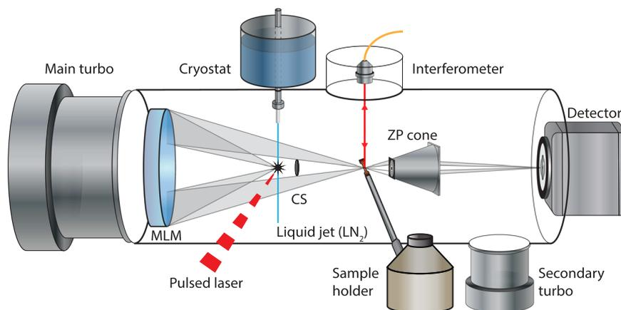
**FIG. 1.** Stability measurement setup in the Stockholm laboratory x-ray cryo microscope. The interferometric sensor head, used for the displacement measurements, was mounted inside the vacuum of the microscope, directly above the sample (shown here) or the zone plate cone. Two turbo pumps can be seen directly connected to the vacuum chamber.
