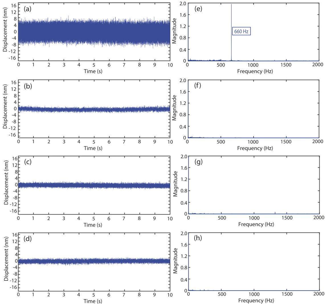
**FIG. 3.** Stability measurements on the zone plate cone. The displacement plots in the time domain are shown in the left column, and the corresponding spectra in the frequency domain are shown to the right. Four separate measurements are presented: With the main turbo pump connected to the microscope chamber and turned on [(a) and (e)] and off [(b) and (f)]. With the main turbo pump decoupled from the microscope chamber and turned on [(c) and (g)] and off [(d) and (h)].
