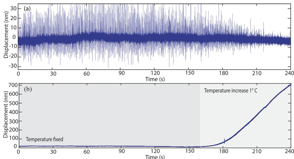
**FIG. 5.** Long-term displacement measurements on the cryo sample holder. Both results are presented during 240 s. (a) A large vibration amplitude caused by high evaporation of liquid nitrogen, a minute after refilling cryo sample holder. (b) Constant displacement (within  $<5$  nm) of the cryo sample holder, kept at  $-168.4$  °C. After 160 s, a small change in the temperature (1 °C) caused a rapid drift.
