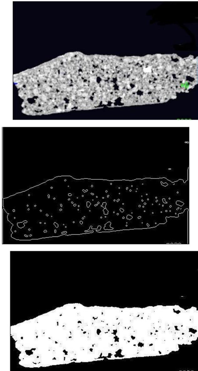
**Figure 12.** (a) Part three of the sample investigation by CT of the Coptic mural painting from the monastery of St Simeon in Aswan). (b) Black areas show porosity and contain gaps. CT image showing the surface as white areas with porosity areas in black indicating the loss of most of the surface and the major composites.
