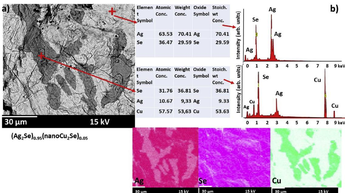
Fig. 2. SEM micrograph (a) and EDX elemental analysis (b) of  $(\text{Ag}_2\text{Se})_{0.95}(\text{Cu}_2\text{Se})_{0.05}$  sample showing the composite nature of the material.
