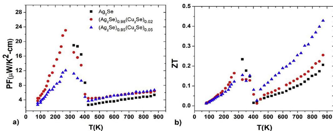
Fig. 8. (a) Thermoelectric figure of merit (ZT) and (b) Power factor versus temperature for  $(\text{Ag}_2\text{Se})_{1-x}(\text{Cu}_2\text{Se})_x$  samples, where  $x = 0, 0.02$  and  $0.05$ .
