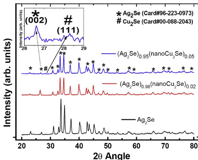
Fig. 1. PXRD pattern of (Ag<sub>2</sub>Se)<sub>1-x</sub>(Cu<sub>2</sub>Se)<sub>x</sub> samples, where x = 0, 0.02 and 0.05.
