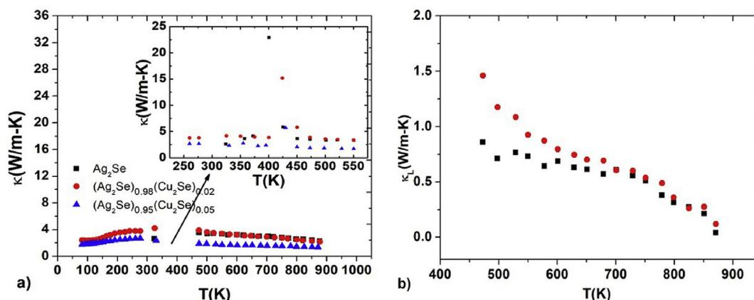
Fig. 7. Total thermal conductivity (a) and lattice part of the thermal conductivity (b) versus temperature for  $(\text{Ag}_2\text{Se})_{1-x}(\text{Cu}_2\text{Se})_x$  samples, where  $x = 0, 0.02$  and  $0.05$ . The  $x = 0$  sample is not included in (b) due to the unphysical negative values of the lattice thermal conductivity, as explained in the text.
