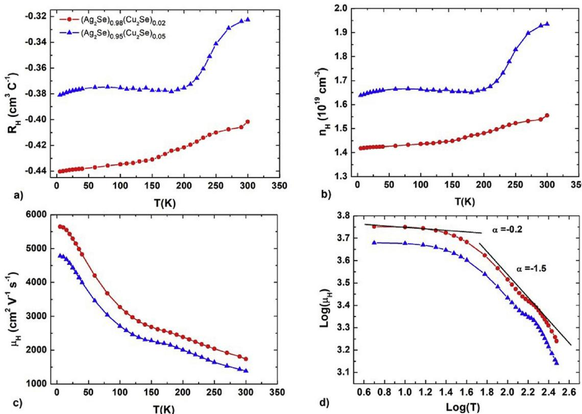
Fig. 5. Temperature-dependent a) Hall coefficient, b) carrier density, c) carrier mobility and d) log mobility vs log temperature for  $(\text{Ag}_2\text{Se})_{1-x}(\text{Cu}_2\text{Se})_x$  samples, where  $x$  is 0.02 and 0.05.
