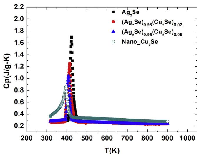
Fig. 4. Temperature dependence of heat capacity for  $(\text{Ag}_2\text{Se})_{1-x}(\text{nano-Cu}_2\text{Se})_x$  and nano  $\text{Cu}_2\text{Se}$  samples, where  $x = 0, 0.02$  and  $0.05$ .
