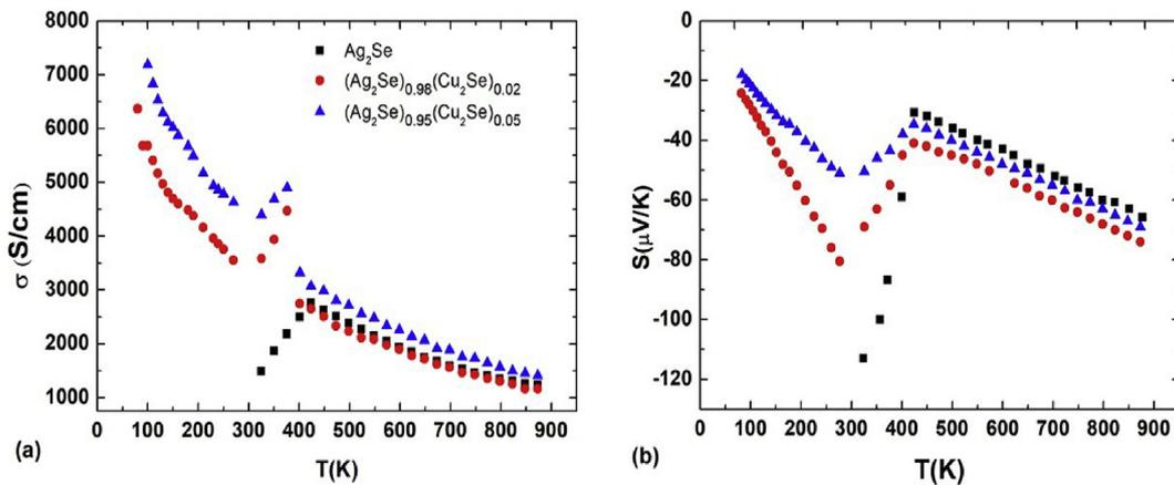
Fig. 6. Temperature-dependent electrical conductivity (a) and Seebeck coefficient (b) of  $(\text{Ag}_2\text{Se})_{1-x}(\text{Cu}_2\text{Se})_x$  samples, where  $x = 0, 0.02$  and  $0.05$ .
