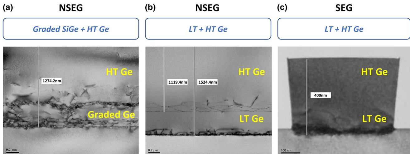
**Fig. 3** Cross-section TEM images of the **a** graded SiGe grown on Si substrate, **b** two-step Ge grown on Si substrate, **c** two-step Ge grown on patterned SOI substrate using selective epitaxial growth
