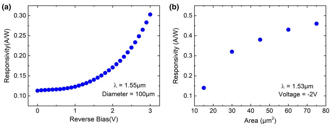
**Fig. 6** **a** Responsivity versus reverse bias for the NSEG Ge PIN detector with a diameter of 100  $\mu\text{m}$ , and **b** responsivity versus area for the SEG Ge PIN detector under the voltage of  $-2$  V
