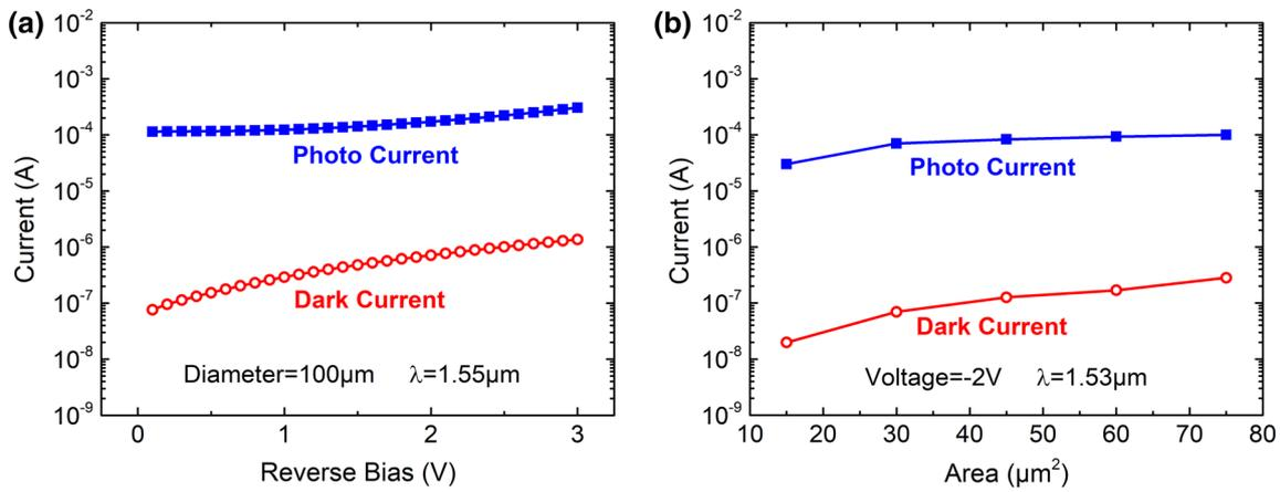
**Fig. 5** **a** Current–voltage characteristic of the 100- $\mu\text{m}$ -diameter device under illumination of 1550 nm light and **b** current–area characteristic of the device under the illumination of 1530 nm light
