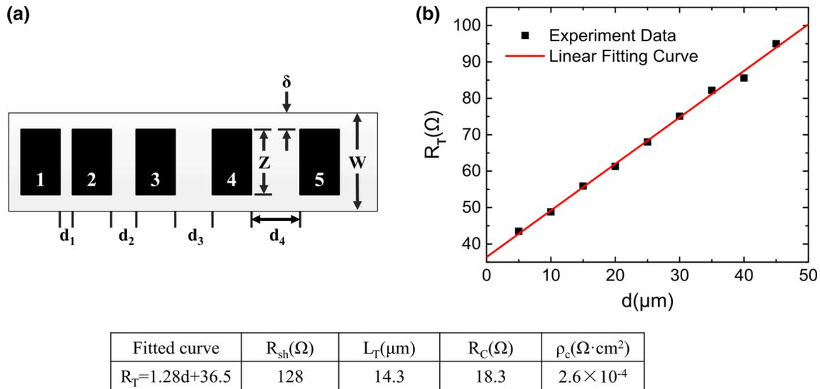
Fig. 7 a Chip layout of TLM mask, b resistance versus the pad distances
