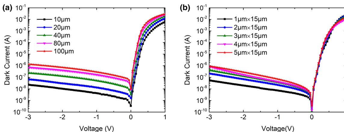
**Fig. 4** Dark current of PDs with different areas **a** NSEG detectors with diameters of 10, 20, 40, 80, and 100  $\mu\text{m}$  and **b** SEG filled trenches 15  $\mu\text{m}$  long and: 1, 2, 3, 4, and 5  $\mu\text{m}$  wide
