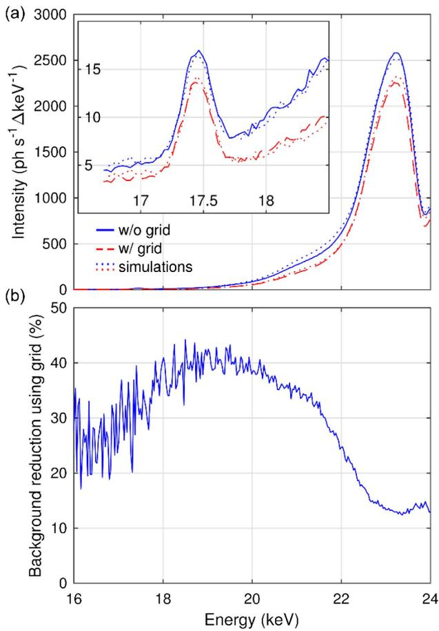
**Fig. 2.** (a) Measured and simulated spectra with and without the anti-scatter grid. The inset shows an enhanced view over the XRF signal. (b) Background reduction using the anti-scatter grid as a function of energy.
