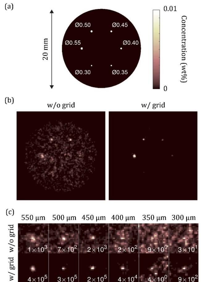
**Fig. 3.** (a) Phantom used for tomography simulations. It is a 20 mm diameter PET cylinder with six holes, 300–550  $\mu\text{m}$ , filled with a 0.01 wt. % Mo solution. (b) Reconstructed images of a tomography without and with an optimized anti-scatter grid. (c) Comparison of the reconstructed signal. The numbers are the  $\text{SNR}^2$  calculated according to the Rose criterion.
