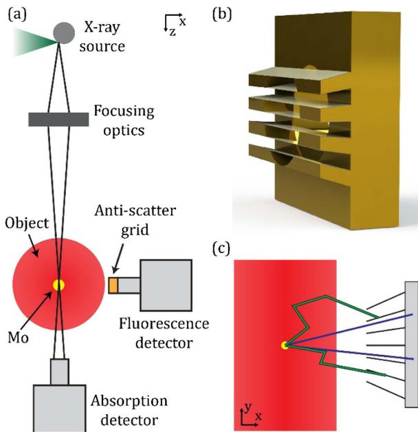
**Fig. 1.** (a) Overview of the imaging system. (b) 3D rendering of the anti-scatter grid. The grid consists of seven tungsten grid bars supported by a copper baseplate. (c) Side view of the object and anti-scatter grids. Multiple scattered photons (green) are blocked by the grid, while the primary photons (blue) enter the detector.
