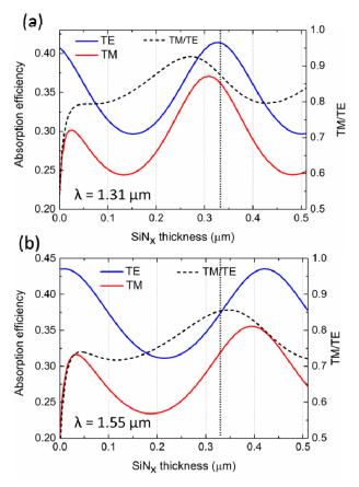
Fig. 4. Calculated dependence of TE and TM absorption efficiency, as well as the TM/TE absorption ratio, as a function of the thickness of the  $SiN_x$  cap layer at (a) 1.31  $\mu$ m, and (b) 1.55  $\mu$ m.
