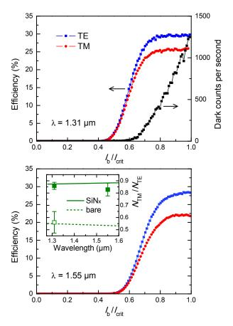
Fig. 5. Detection efficiency as a function of the bias current / critical current ratio ( $I_b/I_{crit}$ ), measured for a typical SNSPD device (a) at 1.31  $\mu m$ , and (b) at 1.55  $\mu m$ . The dark count rate is represented in (a). Inset in (b): measurement of the  $N_{TM}/N_{TE}$  response ratio of bare devices (open symbol) and devices capped with SiN<sub>x</sub> (solid symbols). The curves represent theoretical calculations for both cases.
