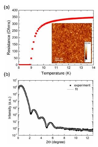
Fig. 1. (a) Film resistance vs. temperature for the NbN thin film under study. Inset:  $1 \times 1 \mu m2$  atomic force microscopy image of the NbN surface. (b) X-ray reflectivity of the NbN film on SiO2-on-silicon. Black squares are experimental measurements and the solid gray line is a fit generated with the GenX software.
