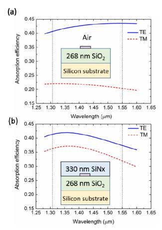
Fig. 3. Calculated absorption efficiency as a function of the wavelength (a) for the uncapped NbN meander; (b) for the NbN meander covered with 330 nm of SiN<sub>x</sub>. Insets: Designs of the structures for which simulations have been performed.
