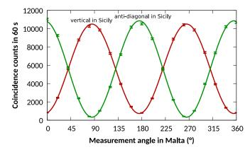
**Fig. 3.** Coincidence count rates for one detector pair and two different measurement angles in Sicily [V (red) and A (green)] as a function of the measurement angle for the analyzer in Malta,  $\phi_M$ , starting from H (red) or D (green). Poissonian statistics are assumed for the data as indicated by the error bars.
