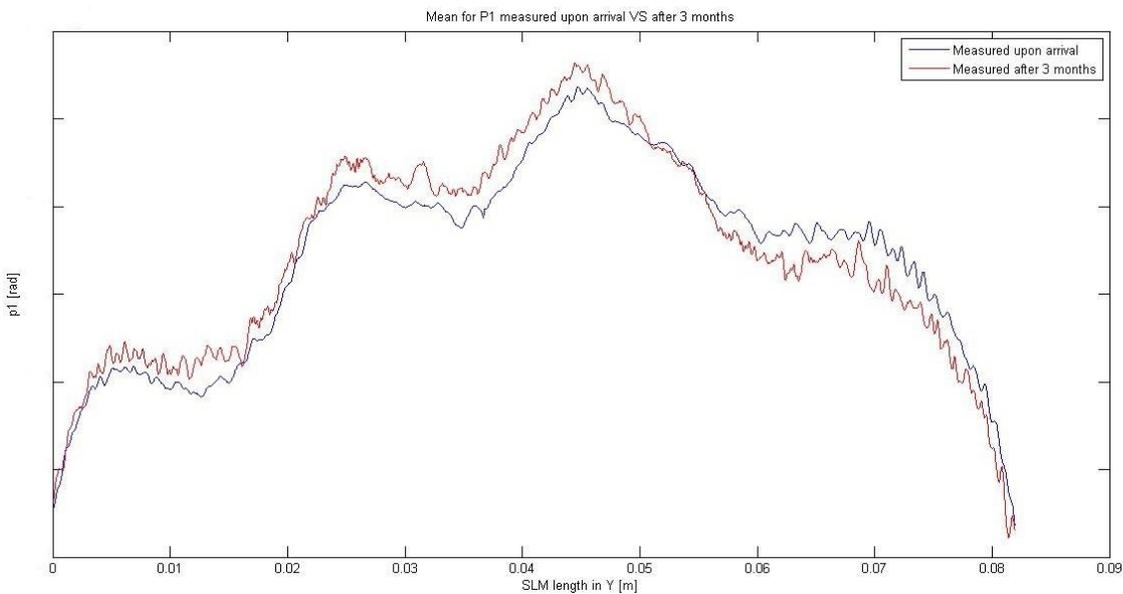
**Figure 38** Plots displaying the mean values for P1 along the length of the SLM measured upon delivery at Micronic Mydata and after three months.
