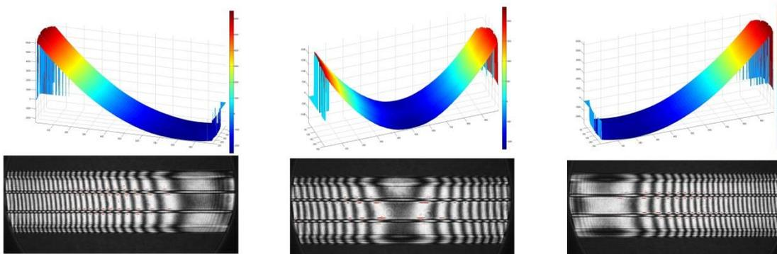
**Figure 17** Three plots of the same surface of an SLM showing different results depending on which part of the SLM is parallel to the Fisba.
