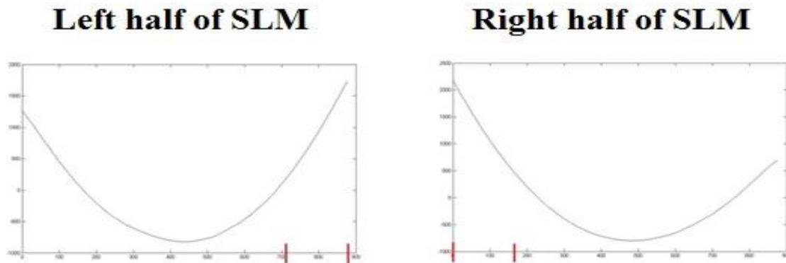
**Figure 18** *Plots displaying the average value along the length of an SLM where the X-axis represents measured points and Y-axis average height variation in nanometers. The red marks on the X-axis represent the boundaries of the overlapping areas.*
