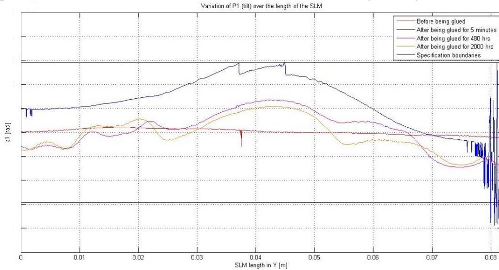
**Figure 55** The plot above shows the parameter P1 before and after the SLM had been glued.
