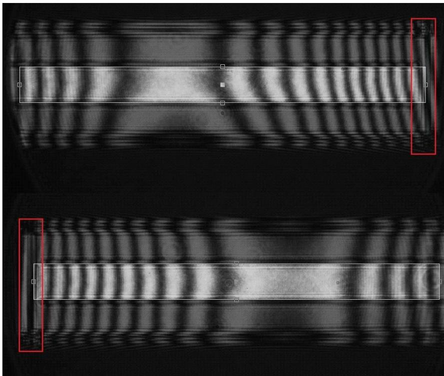
**Figure 15** Screenshot from  $\mu$ Shape Professional showcasing the fit of the measurement masks.
