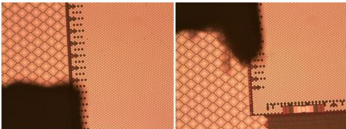
**Figure 13** Pictures from the Leica INM 100 of the short end of the SLM with the Post-It fixed at the border of the active area of the mirrors.
