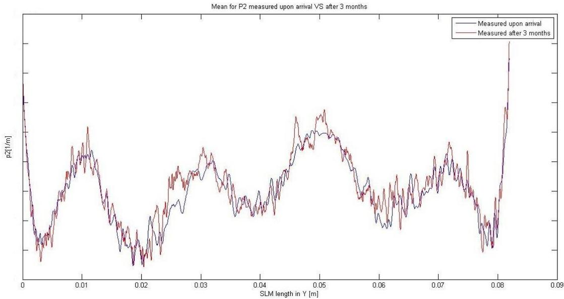
**Figure 33** *Plots for stability verification displaying the mean values of P2 along the length of the SLM measured upon delivery at Micronic Mydata and after three months.*
