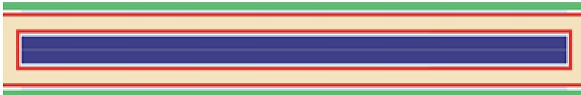
**Figure 9** *The image above represents an SLM seen from a top side view where the blue area represents the area of interest (active mirrors).*
