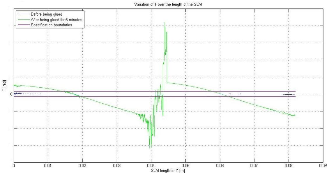
**Figure 54** The plot above shows the parameter *T* before and after the SLM had been glued.
