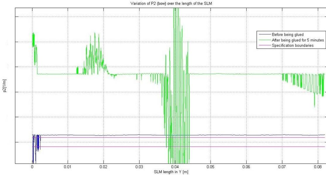
**Figure 53** The plot above shows the parameter *P2* before and after the SLM had been glued.
