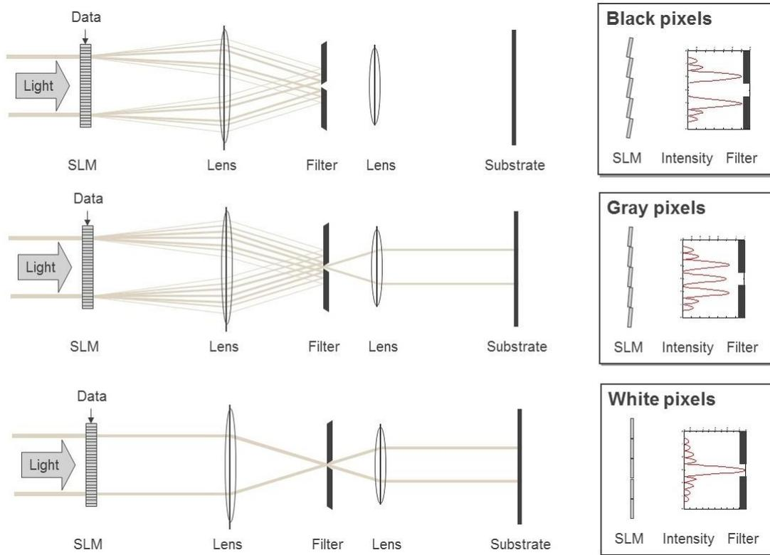
**Figure 4** The figures above show how the light intensity is seen at the filter resulting in the according color at the substrate. [1]
