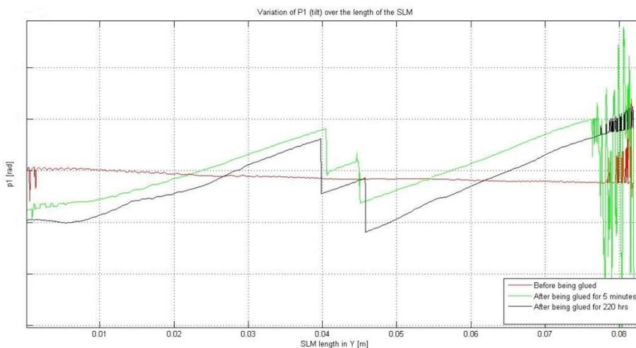
**Figure 43** The plot above shows the parameter P1 before and after the SLM had been glued.
