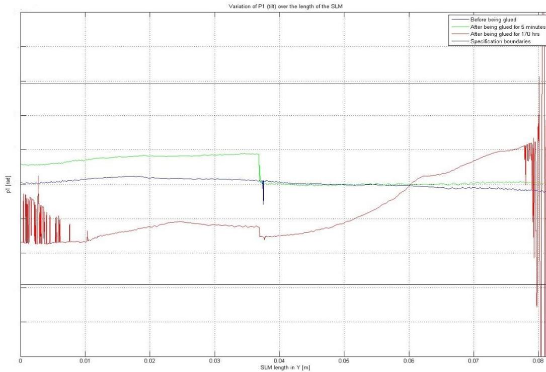
**Figure 49** The plot above shows the parameter P1 before and after the SLM had been glued.
