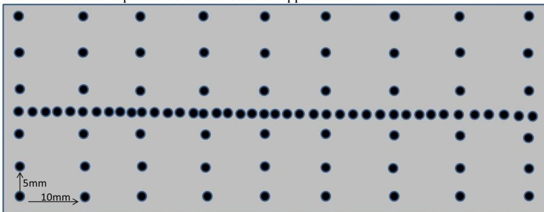
**Figure 25** *The figure above displays the pattern chosen to measure the aluminum blocks used for the experiments. The distance between the horizontally placed measurement points in the middle of the block was 2mm.*
