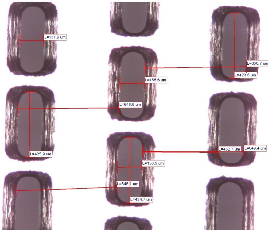
Figure 27 Picture taken using the Leica 100 of the shadow mask used as a mesh for applying the adhesive.
