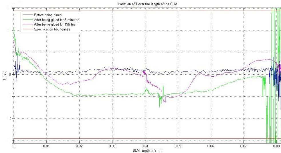
**Figure 45** The plot above shows the parameter T before and after the SLM had been glued.
