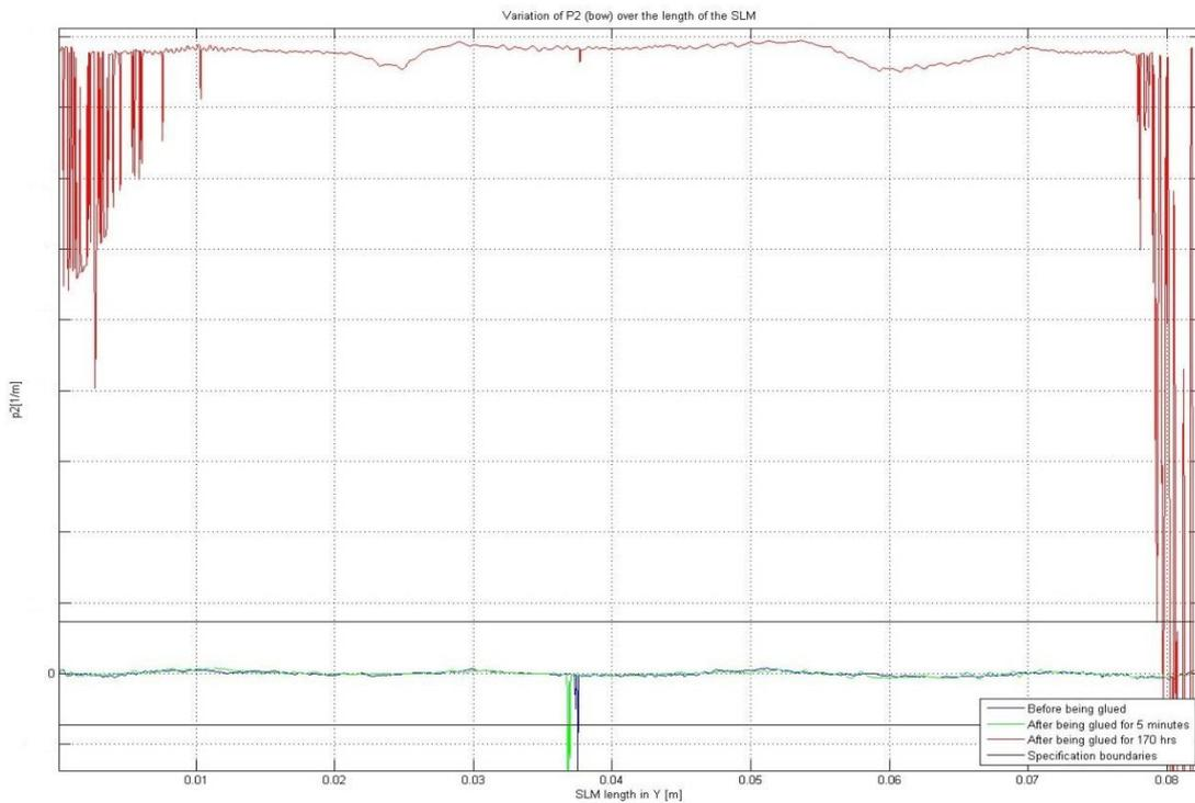
**Figure 50** The plot above shows the parameter P2 before and after the SLM had been glued.
