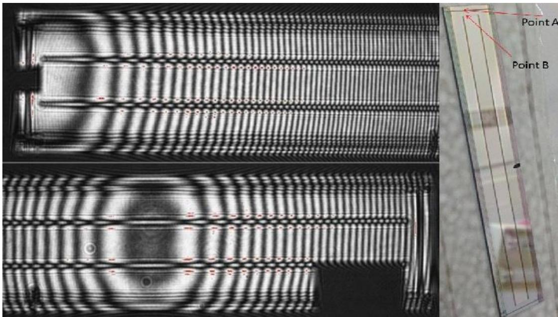
**Figure 14** *The top left picture shows the SLM with the Post-It attached to the short end. The bottom left picture below shows the SLM with the Post-It attached to the long end. Picture to the right displays the newly chosen reference point in relation to the edge on the short end of the zone of active mirrors.*
