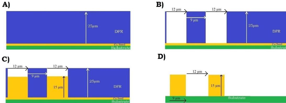
**Figure 2** The figures above briefly show the process flow for obtaining the desired patterns on a substrate using the LDI.
