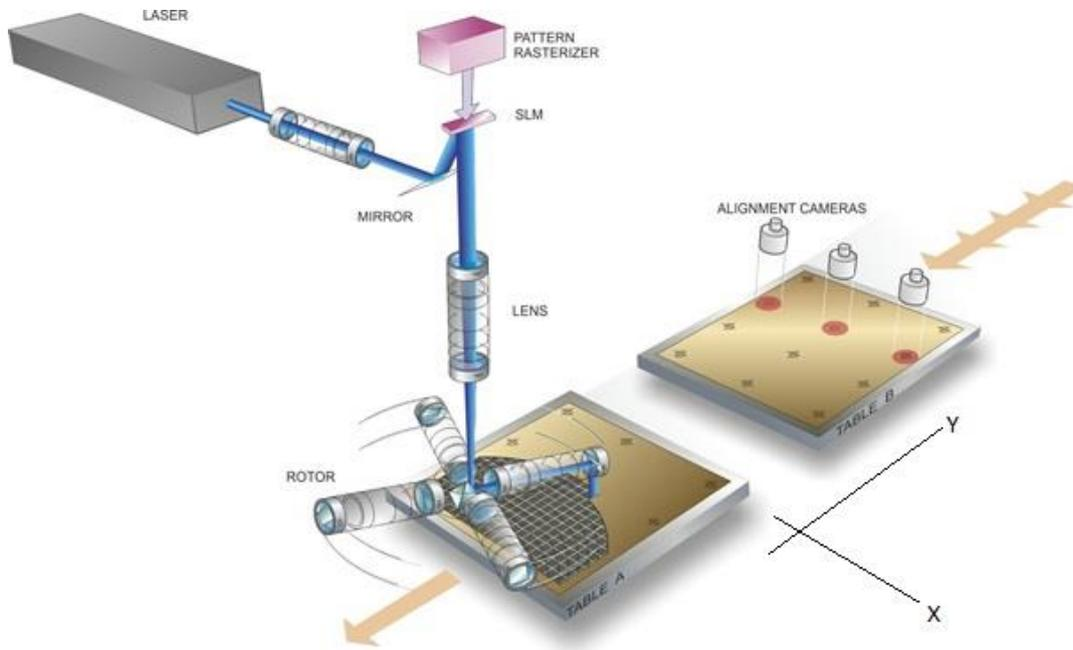
*Figure 1 High level schematic for how the LDI pattern generator works. [1]*
