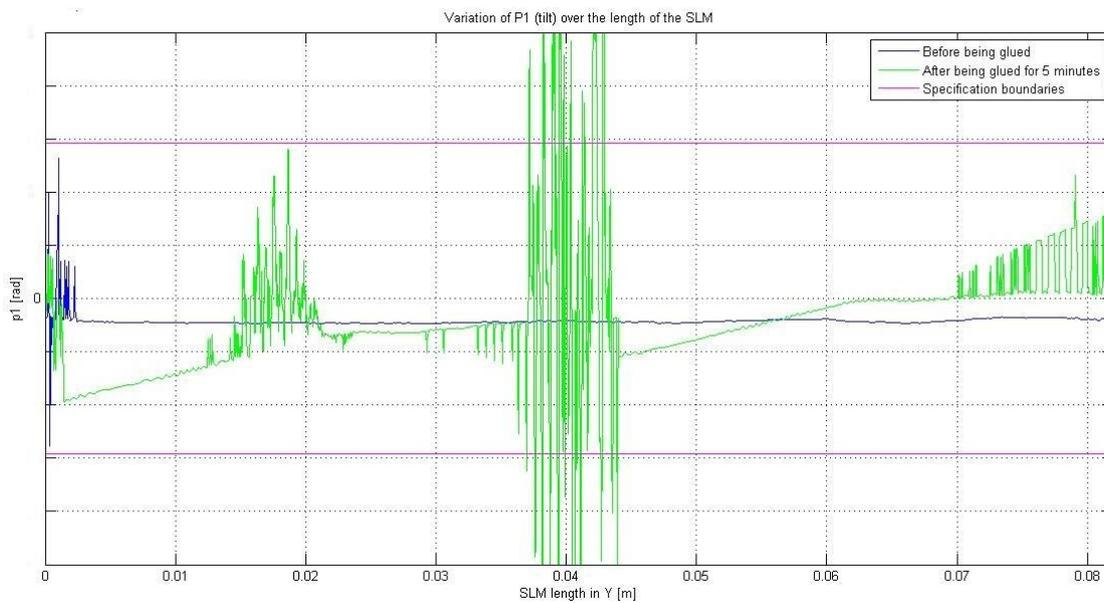
**Figure 52** The plot above shows the parameter  $P1$  before and after the SLM had been glued.
