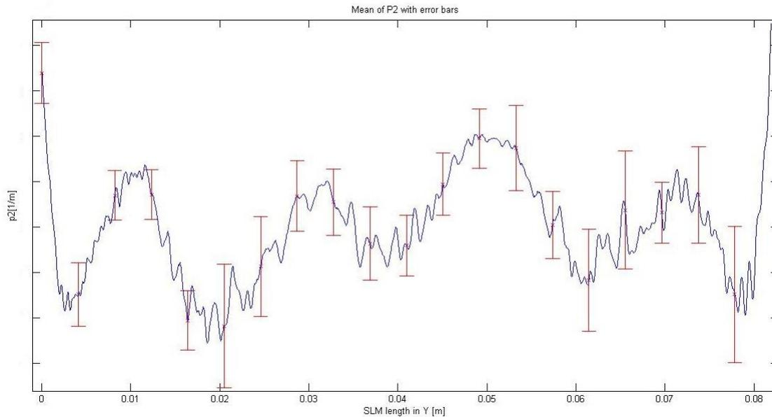
**Figure 31** Mean value of P2 with error bars representing the standard deviation.
