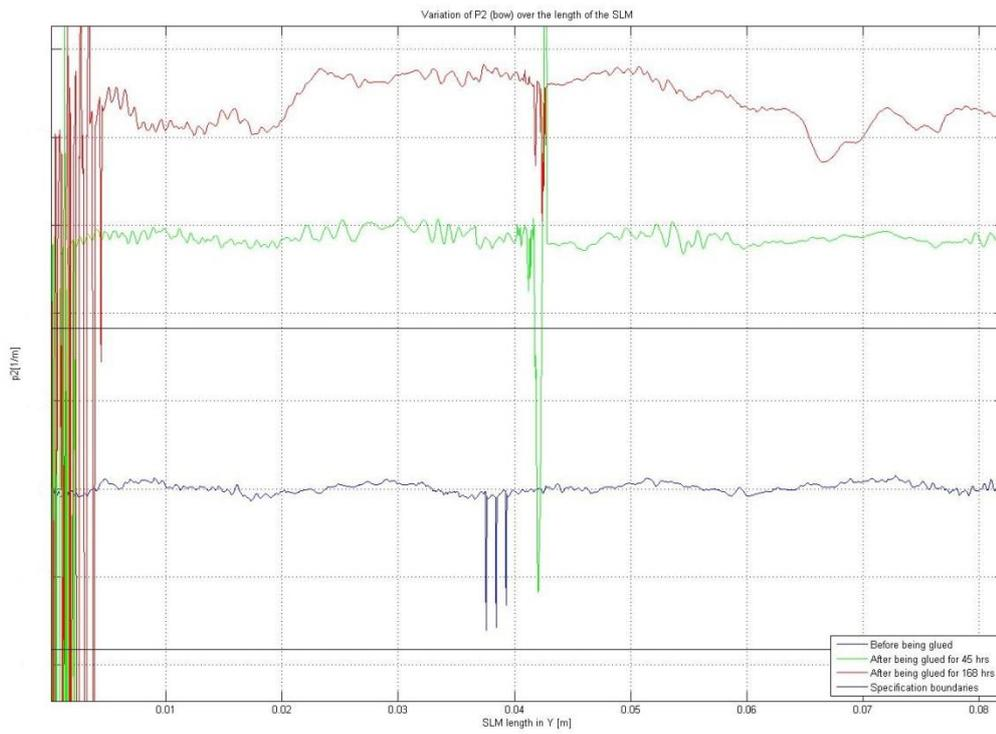
**Figure 47** The plot above shows the parameter P2 before and after the SLM had been glued.
