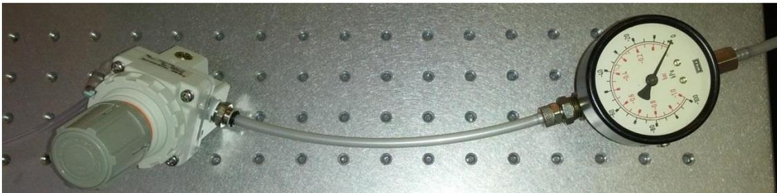
**Figure 29** Pressure regulator and vacuum gauge.
