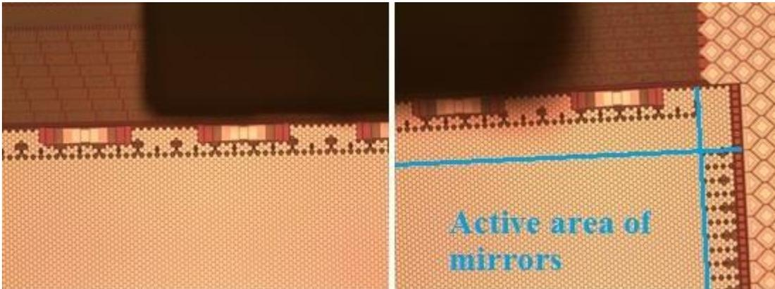
**Figure 12** Pictures from the Leica INM 100 of the long end of the SLM with the Post-It fixed at the border of the active area of the mirrors.
