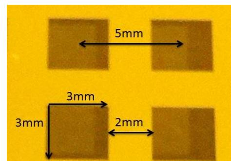
*Figure 23 Dimensions of squares on the Mix N Match mask.*
