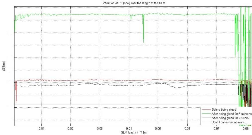
**Figure 44** The plot above shows the parameter P2 before and after the SLM had been glued.
