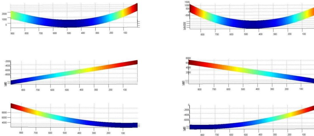
**Figure 20** *On the left are plots representing one half of an SLM and on the right are plots representing the other half of the same SLM. The plots at the top display the data sets before any manipulation has been performed. The plots in the middle display the matrixes representing the lean between the boundaries of the overlapping area. The plots at the bottom display the data sets after the rotation has been performed.*
