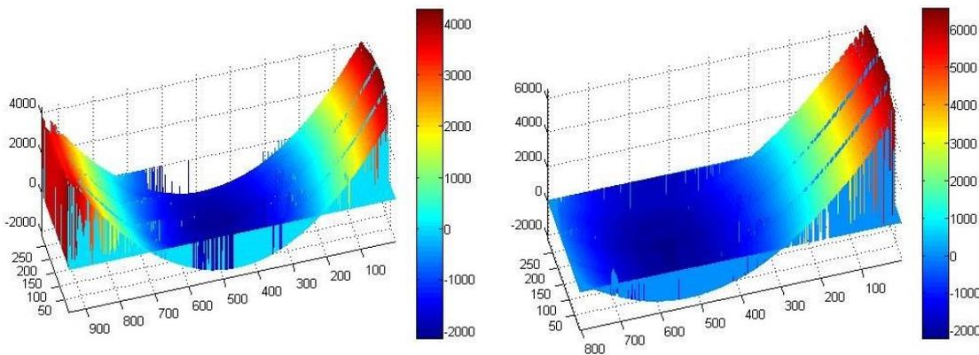
**Figure 10** Representation of the height variation in two data sets of the same SLM with an overlapping area (X-label and Y-label display measured points and the Z-axis displays the height variation in nanometers).
