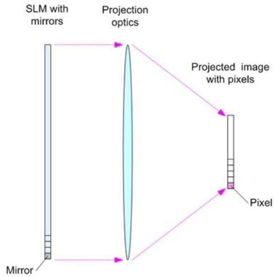
**Figure 3** The pattern generated by the SLM decreases in size when projected. [1]
