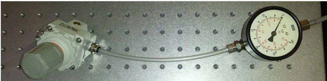
**Figure 29** *Pressure regulator and vacuum gauge.*
