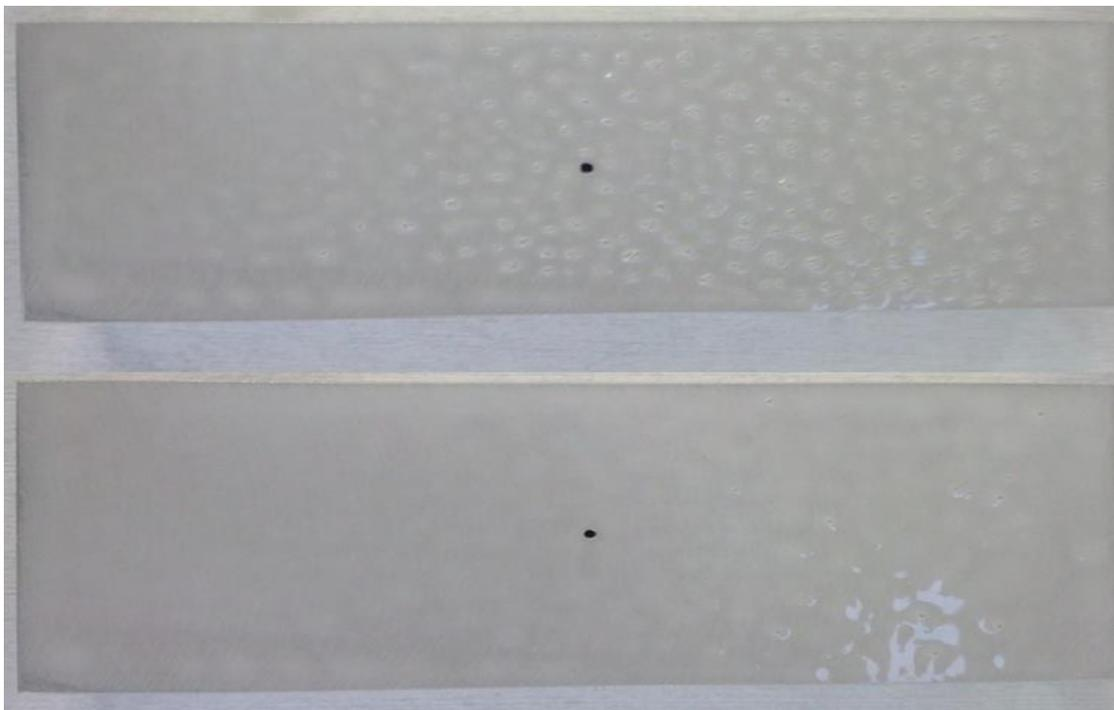
**Figure 26** *Top picture shows the air bubbles in the adhesive just after removing the mesh. The bottom picture shows that after 8 minutes most of the air bubbles had disappeared. The black dot at the center of the block is the vacuum hole.*
