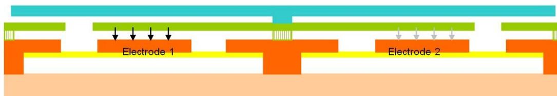
**Figure 5** Cross section of an SLM mirror. [2]
