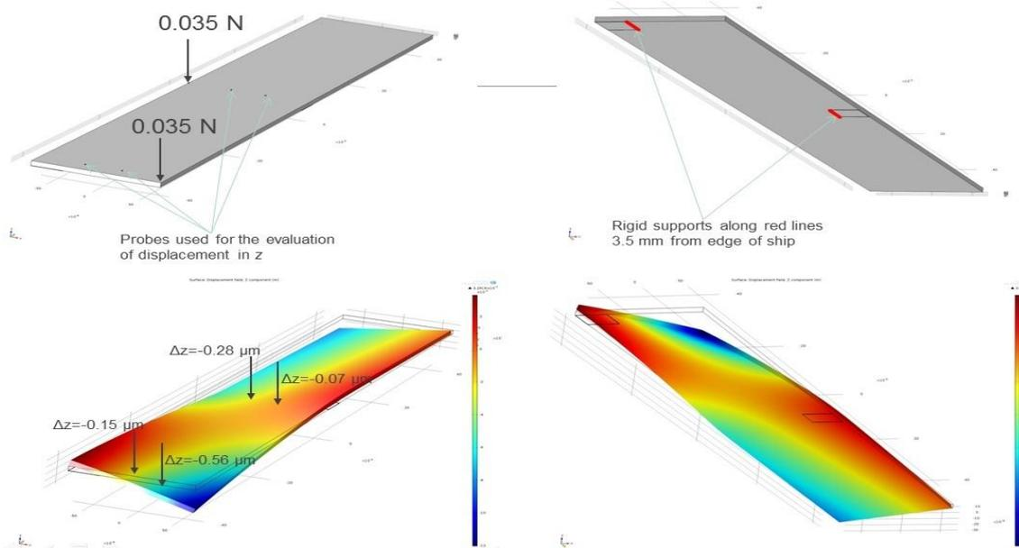
**Figure 41** Simulation plots from Comsol Multiphysics.
