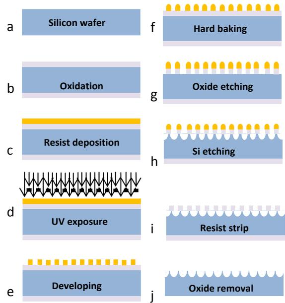
Figure 4.4 Schematic of the fabrication process.
