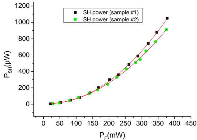
Figure 6.10 The SH power versus the fundamental power in 2 different samples with 5  $\mu\text{m}$  grating period. Solid squares and circles are experimental data and red solid line is the theoretical curve.
