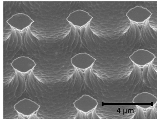
Figure 4.20 SEM image of 5  $\mu\text{m}$  period pattern.
