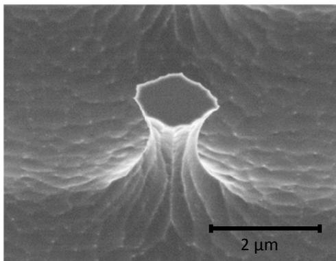
Figure 4.19 SEM image of a needle in 5  $\mu\text{m}$  period pattern with height of 2.8 and top diameter of approximately 2  $\mu\text{m}$
