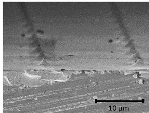
Figure 4.18 SEM image of 20  $\mu\text{m}$  period pattern.
