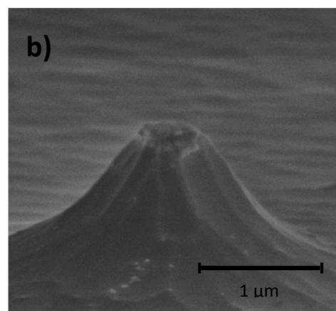
Figure 6.2 SEM picture of a needle in  $20 \mu\text{m}$  period a) before and b) after poling. The tip diameter increases from  $50 \text{ nm}$  to  $500 \text{ nm}$  during contacting silicon chip and crystal.
