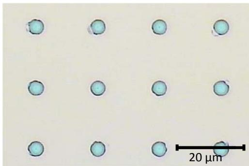
Figure 4.13 Optical microscope image of 20  $\mu\text{m}$  period pattern after lithography.
