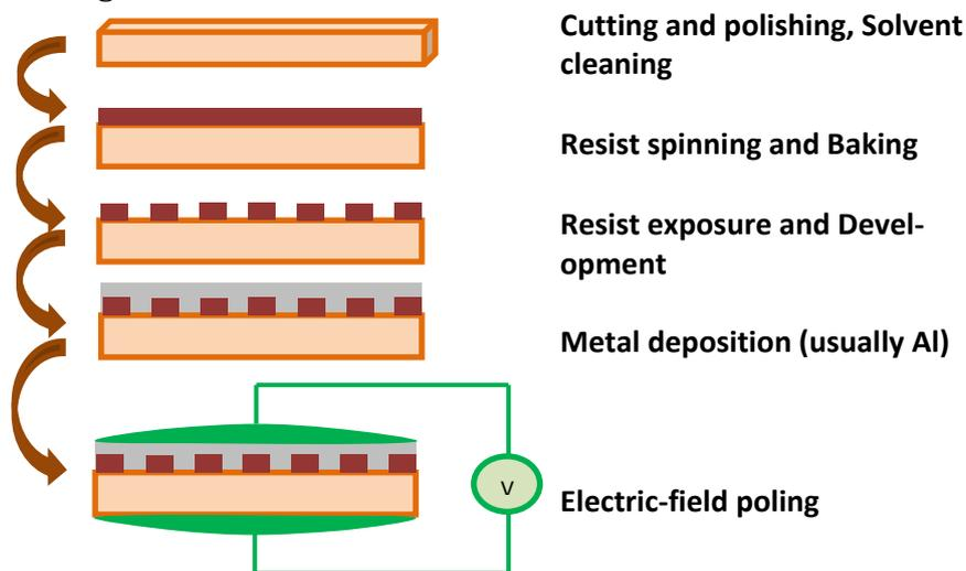
Figure 2.3 Contact electrode poling process.
