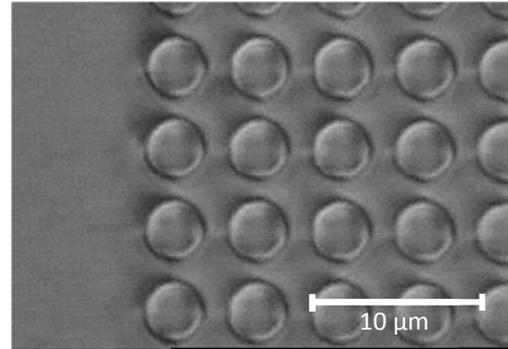
Figure 4.6 Optical microscope image of 5  $\mu\text{m}$  period pattern after oxide etching.
