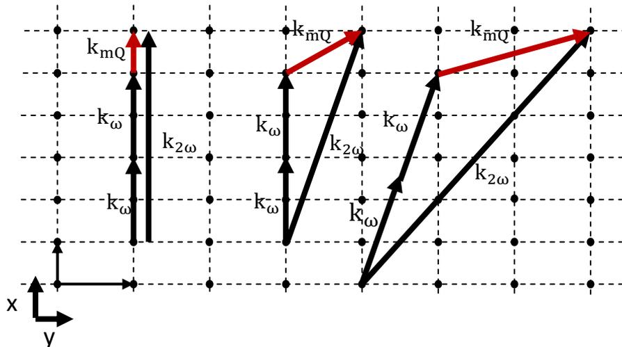
Figure 2.4 Possible  $k$ -vectors for compensating phase mismatch in a 2D QPM crystal.
