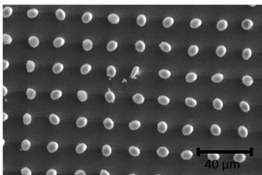
Figure 4.15 SEM image of 20  $\mu\text{m}$  period pattern after isotropic Si etch.
