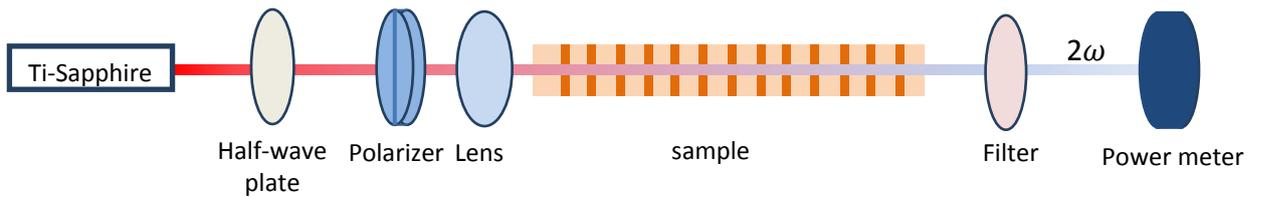
Figure 6.8 SHG setup for measuring conversion efficiency.
