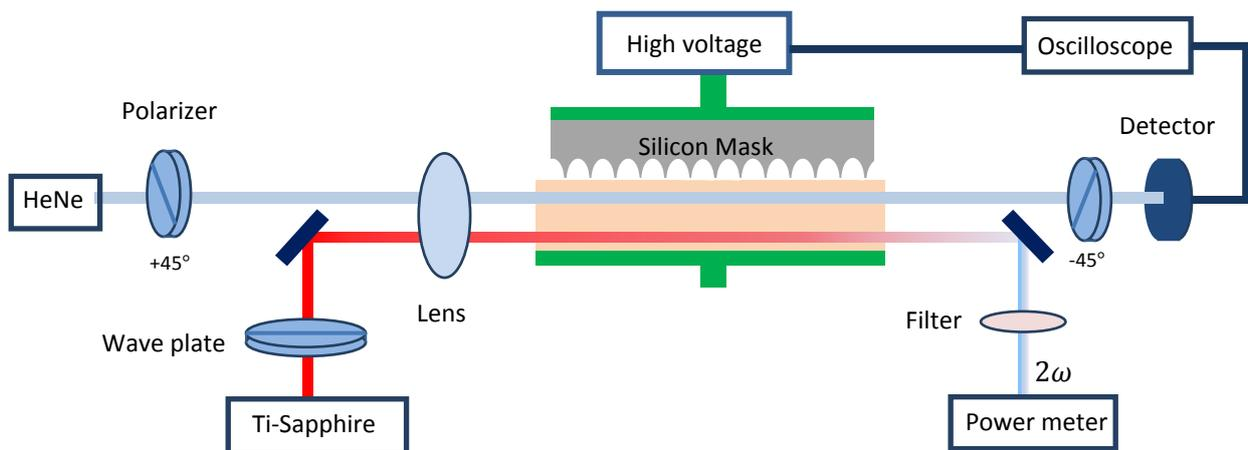
Figure 5.3 Poling monitoring setup.
