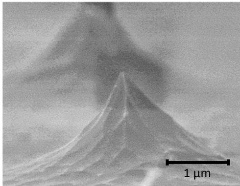
Figure 4.17 SEM image of a needle in 20  $\mu\text{m}$  period pattern with height of 1.73 and tip diameter of 50 nm.
