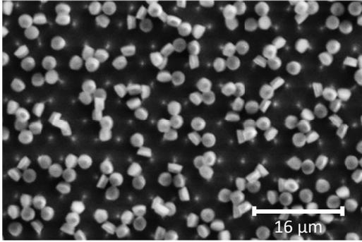
Figure 4.11 SEM image of 3.2  $\mu\text{m}$  period pattern after isotropic Si etch, masks drop.
