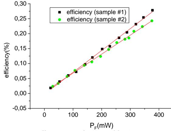
Figure 6.9 The SHG conversion efficiency as a function of fundamental power for 2 samples with 5  $\mu\text{m}$  grating period. Circles and squares are measured data and red lines are linear fits, respectively.
