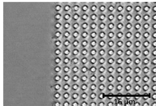
Figure 4.10 Optical microscope image of 3.2  $\mu\text{m}$  period pattern after oxide etching.
