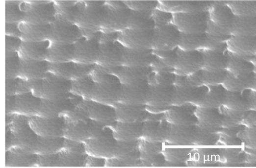
Figure 4.12 SEM image of 3.2  $\mu\text{m}$  period pattern after mask removal, over etched pattern.
