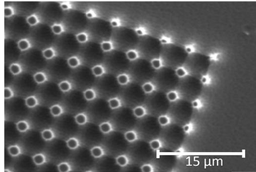
Figure 4.8 SEM image of 5  $\mu\text{m}$  period after mask removal, formation of plateaus.
