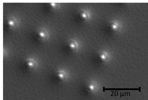
Figure 4.16 SEM image of 20  $\mu\text{m}$  period pattern after mask removal, needles are formed.
