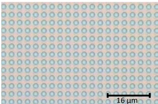
Figure 4.9 Optical microscope image of 3.2  $\mu\text{m}$  period pattern after lithography.
