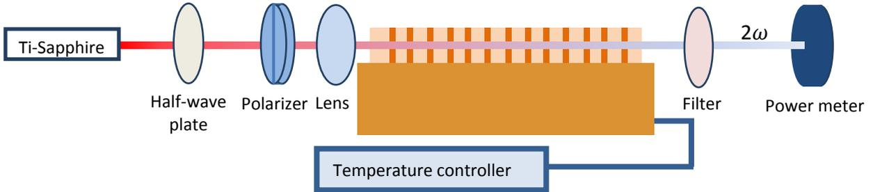
Figure 6.11 Temperature tuning setup for SHG.
