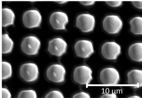
Figure 4.7 SEM image of 5  $\mu\text{m}$  period pattern after isotropic Si etch.
