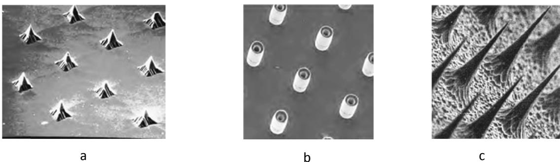
Figure 4.1 Various types of silicon needles obtained by different techniques [33] , [34] , [35].
