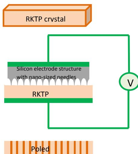
Figure 5.1 Schematic of poling technique with silicon electrodes.
