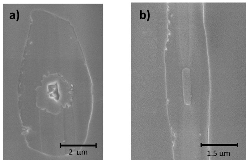
Figure 6.4 SEM pictures of domains formed by a sharp spike. (a) Outer dimension:  $3 \mu\text{m}$ , inner not inverted area dimension:  $1.5 \mu\text{m}$ , spike scratch dimension:  $450 \text{ nm}$ . (b) Not inverted area inside a domain without any scratch, width:  $200 \text{ nm}$ .
