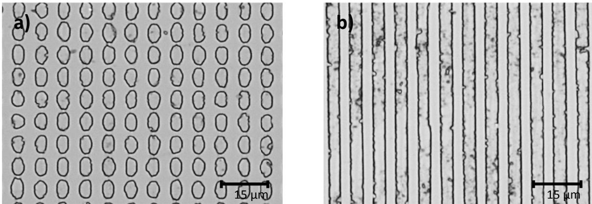
Figure 6.6 Domain structures of poled RKTP sample with 5.4 kV/mm triangular pulse of 3 ms duration and 5 μm grating length. (a)  $C^+$  Domains dimension  $2.5 \times 3.8 \mu\text{m}$  (b)  $C^-$  Domains width 2.6 μm.
