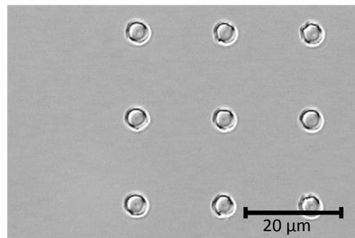
Figure 4.14 Optical microscope image of 20  $\mu\text{m}$  period pattern after oxide etching.
