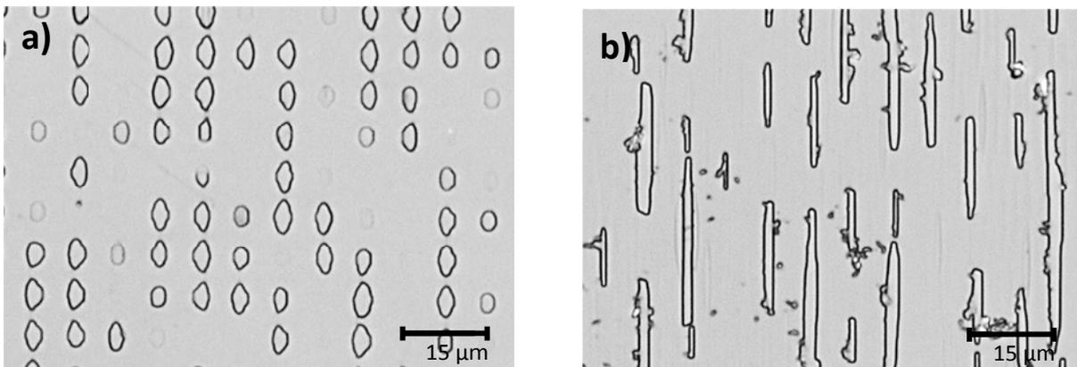
Figure 6.7 Domain structures of poled RKTP sample with 5 kV/mm triangular pulse of 3 ms duration and 5 μm grating length. (a)  $c^+$  Domains dimension  $2 \times 3 \mu\text{m}$  (b)  $c^-$  Domains are distributed randomly width: 1 μm.
