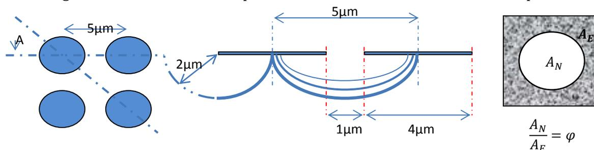
Figure 4.3 Schematic of mask, opening area and ratio of exposed and non-exposed area for a 5  $\mu\text{m}$  period grating.
