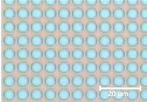
Figure 4.5 Optical microscope image of 5  $\mu\text{m}$  period pattern after lithography.
