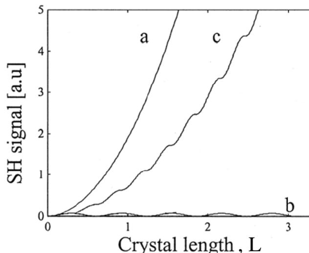
Figure 2.2 Intensity of SHG in different phase matching conditions. a) Perfect phase matching, b) No phase matching and c) Quasi phase matching [14].
