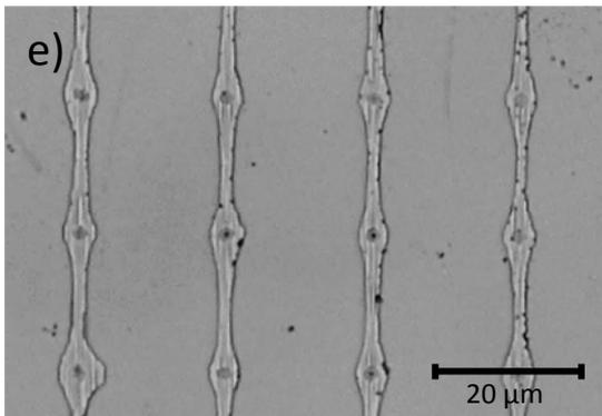
e:  $c^+$  Domain dimension  $5 \mu\text{m}$  at the place of needles,  $1.6 \mu\text{m}$  in between.
