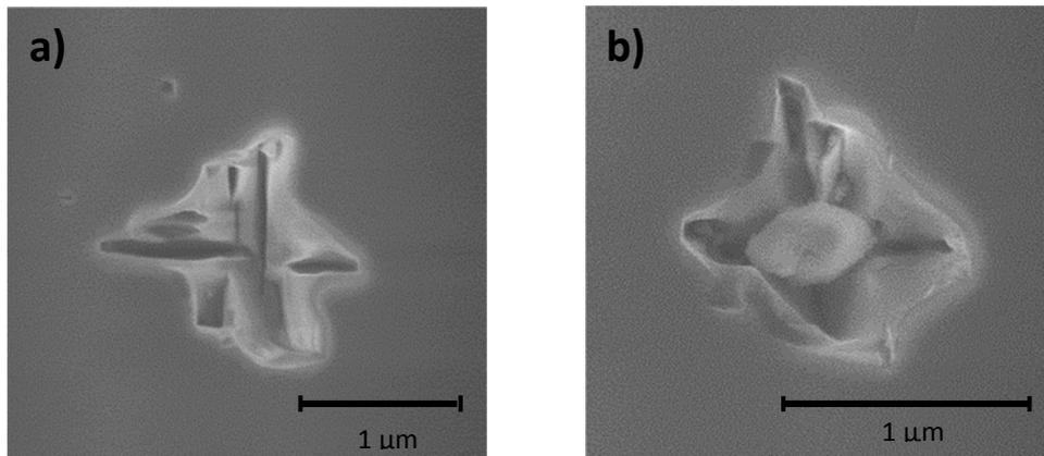
Figure 6.3 SEM pictures of scratches. (a) Scratch of one spike on the crystal surface after alignment. (b) Scratch and broken electrode tip (lying inside) on the RKTP crystal surface.
