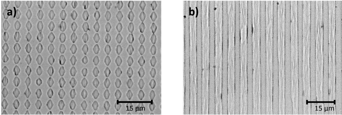
Figure 6.5 Domain structures of poled RKTP sample with 5.4 kV/mm triangular pulse of 3 ms duration and 5 μm grating length. (a)  $c^+$  Domains dimension  $2.5 \times 4.1 \mu\text{m}$  (b)  $c^-$  Domains width 2.5 μm.
