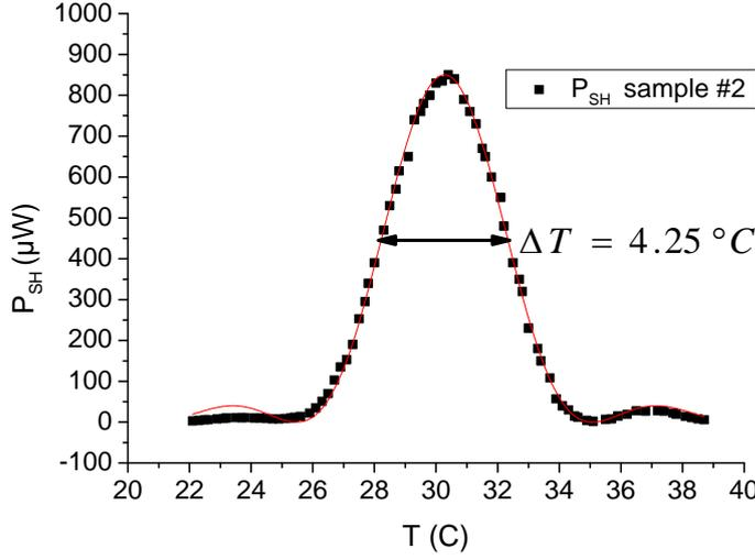
Figure 6.12 Temperature tuning curve for SHG, black squares show observed data and red line is the  $\text{sinc}^2$  fitting function.
