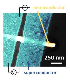
*Hybrid semiconductor nanowire – superconductor device. The scanning electron microscope image shows a nanogap in the nanowire contact electrodes where superconductivity is induced by the proximity effect. A four-point measurement configuration is used for device characterization.*
