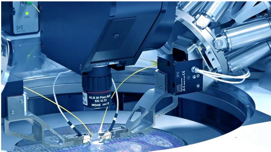
Figure 1. Measurement concept for CMOS circuit testing with quantum sensors: a microscope objective collects infrared light emitted by an integrated circuit under test. This allows for new studies of the circuits performances.
