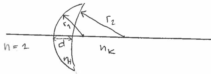
$$\text{Främre styrka: } F_1 = \frac{n_H - n}{r_1} = \frac{1.3771 - 1}{0.0078 \text{ m}} = 48.346 \text{ D}$$
