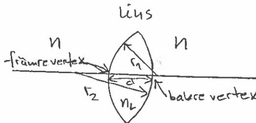
$$\begin{aligned} n_L &= 1.416 & f_1 &= 10.00 \text{ mm} \\ n &= 1.333 & f_2 &= -6.00 \text{ mm} \\ d &= 3.60 \text{ mm} \end{aligned}$$
