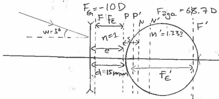
$$\text{Effektiv styrka: } F_E = F_G + F_{\text{öga}} - \frac{d}{n} F_G F_{\text{öga}} = -10 + 68.7 - \frac{0.015}{1} (-10) \cdot 68.7 \\ = 69.0 \text{ D}$$
