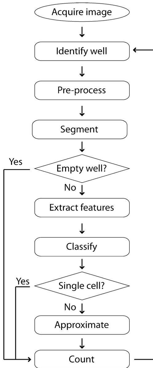
**Fig. 5** Flow chart demonstrating the sequence of steps in the automatic cell counting program. Firstly, the program discriminated between empty and non-empty wells. In non-empty wells individual objects were classified as single cells or clusters, followed by assessment of the number of cells in the clusters and counting. The process was repeated until all wells were analyzed
