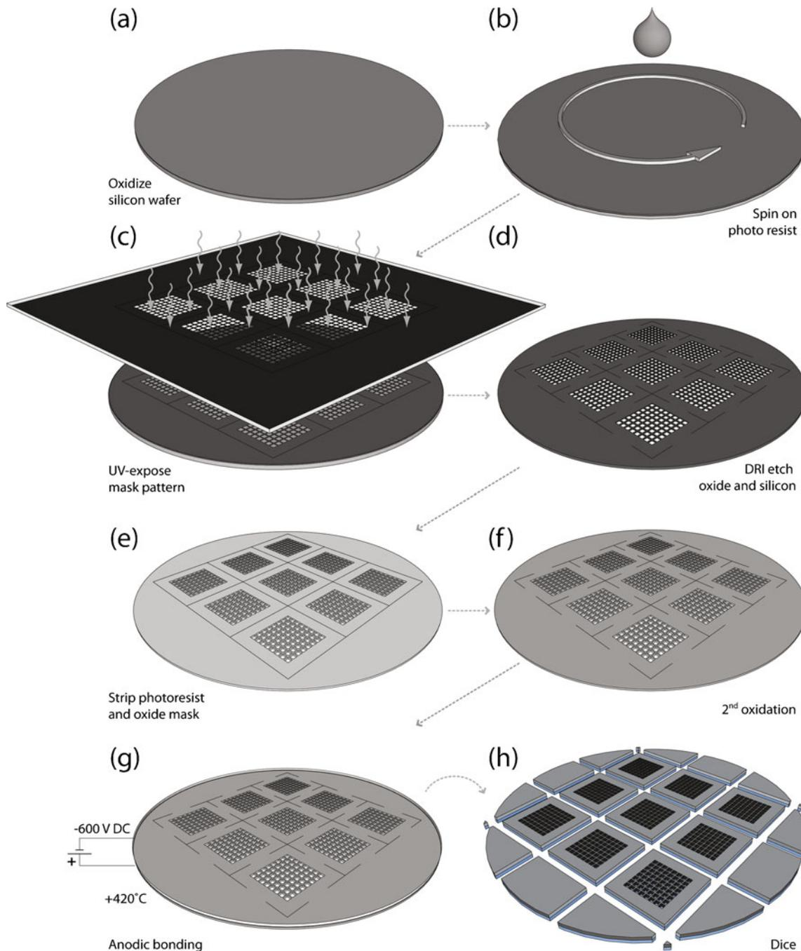
**Fig. 2** Schematic outline of the microchip fabrication process. **(a)** Oxidized silicon wafer. **(b)** Spin coating of wafer with photoresist. **(c)** Masked UV-exposure of photosensitive resist layer. **(d)** Plasma etching of the oxide and silicon. **(e)** Removing photoresist and oxide
