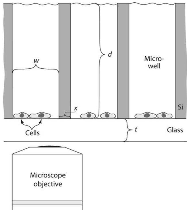
**Fig. 1** Schematic picture showing a cross-section of the microchip. All chips were made from silicon (Si) wafers with a thickness ( $d$ ) of 300 or 500  $\mu\text{m}$ , bonded to glass with a thickness ( $t$ ) of 175  $\mu\text{m}$  allowing imaging with an inverted microscope. The well width ( $w$ ) and wall width ( $x$ ) was varied for the different designs. The sketch is not to scale
