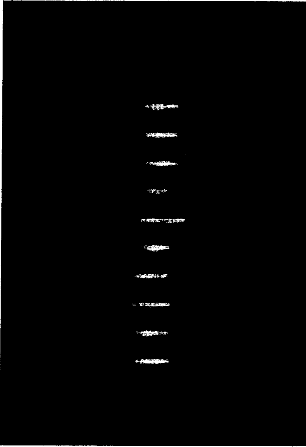
FIG. 2. Photograph of trapped particles in the standing-wave pattern.
