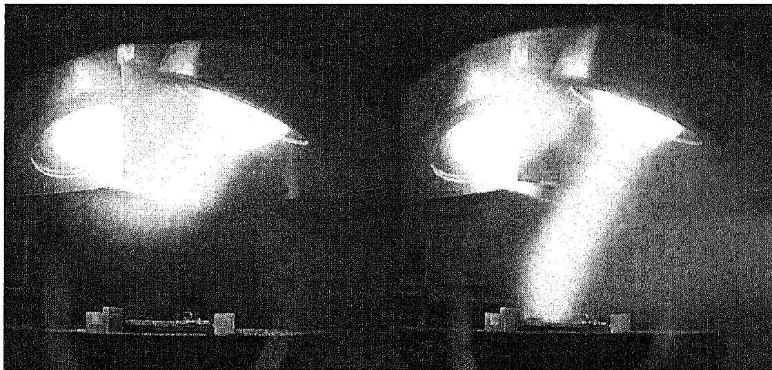
Figure 2: Photograph of the plasma with a solenoid current of 0 A to the left and 5 A to the right. Secondary electrons ejected from the target are guided towards the substrate and the plasma density is clearly enhanced in the substrate region when the solenoid is used.
