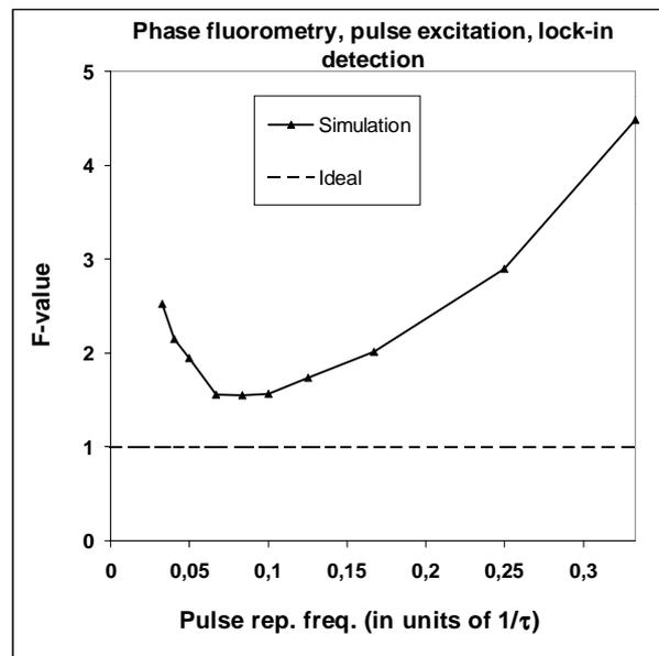
Fig. 10. F as a function of pulse repetition frequency for phase fluorometry with lock-in detection. Smooth, Gaussian-like pulses (see Fig. 9) were used for excitation.
