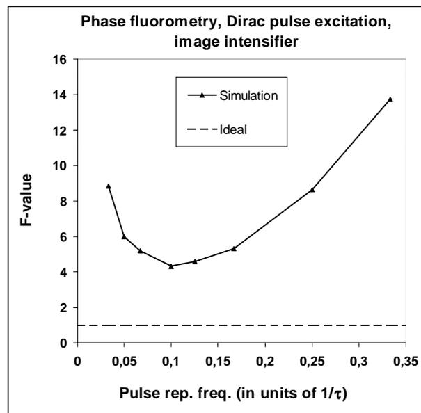
Fig. 4. F as a function of pulse repetition frequency for phase fluorometry using an image intensifier and Dirac pulse train excitation.
