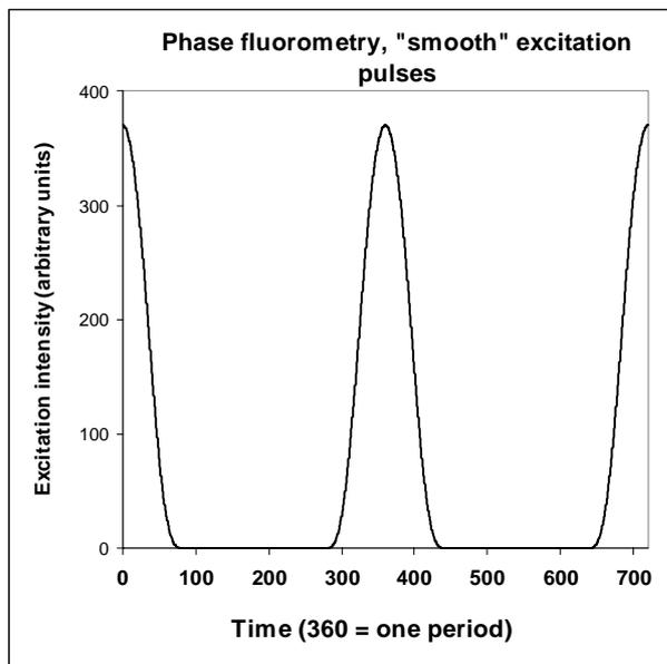
Fig. 9. "Smooth" excitation pulses with a FWHM of 0.2 of one period were simulated to investigate performance when using a non-square-wave pulse train (see text for details)
