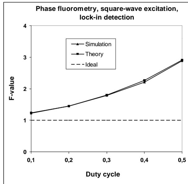
Fig. 8. F as a function of duty cycle for phase fluorometry with lock-in detection. Square-wave pulse excitation with frequency  $0.1/\tau$ , and duty cycles ranging from 0.1 to 0.5.
