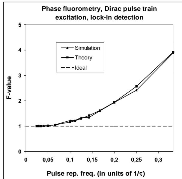
Fig. 6. F as a function of pulse repetition frequency for phase fluorometry with lock-in detection. Dirac pulse train excitation.
