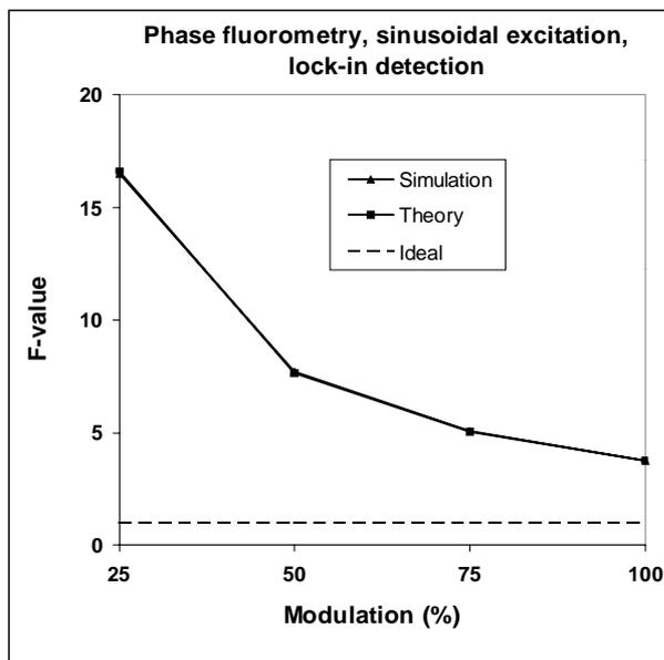
Fig. 11. F as a function of modulation depth for phase fluorometry with lock-in detection. Sinusoidal excitation with frequency =  $0.13/\tau$ .
