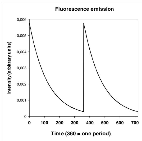
Fig. 1. Fluorescence light intensity as a function of time when using Dirac pulse excitation. Curves like this one were used in the simulations for calculating the probability for fluorophore photon emission.
