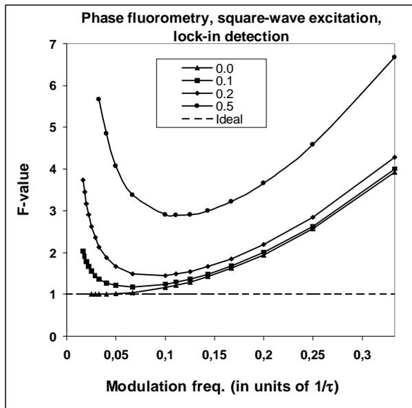
Fig. 7. F as a function of modulation frequency for phase fluorometry with lock-in detection. Theoretical curves are shown for square-wave pulse excitation with duty cycles 0 (= Dirac pulses), 0.1, 0.2, and 0.5. Results from simulations were very close to the theoretical values.
