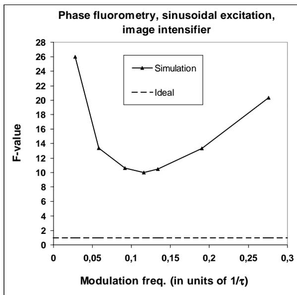
Fig. 3. F as a function of modulation frequency for phase fluorometry, using an image intensifier and sinusoidal excitation.
