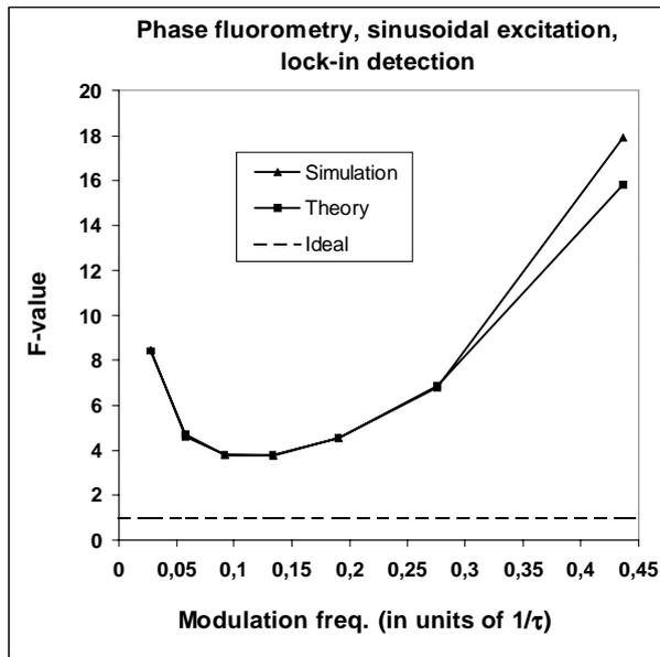
Fig. 5. F as a function of modulation frequency for phase fluorometry with lock-in detection. Sinusoidal excitation.
