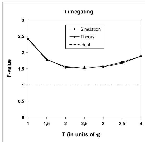
Fig. 2. Figure of merit, F, as a function of window width, T, for timegating (two windows of equal width). Low F-values represent high signal-to-noise ratios. The best F-value theoretically possible is unity.
