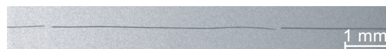
Figure 4. A 10 ns flash photograph of a xenon jet several centimetres from the nozzle orifice. The jet is broken at several locations but no signs of general droplet formation are visible (from [20]).
