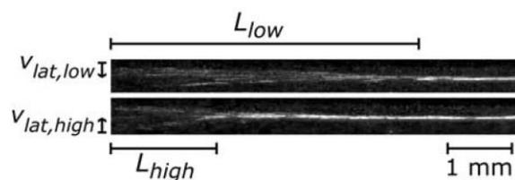
**Fig. 2** High-speed USW alignment of  $10 \mu\text{m}$  fluorescent beads at a mean flow velocity of  $19 \text{ mm s}^{-1}$  and at transducer voltages of  $4 V_{\text{RMS}}$  (top picture) and  $7 V_{\text{RMS}}$  (bottom picture). The corresponding maximum focusing distances ( $L$ ) and lateral mean velocity of beads ( $v_{\text{lat}}$ ) are marked for the low and high transducer voltages.
