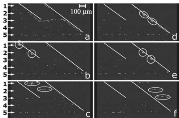
**Fig. 6** Particle switching experiments. Merging of USW lanes by DEP (a). Sideways shifting of lanes (b–f). The arrows mark the five USW pressure node and the solid lines mark the electrodes. The ellipses denote the trajectories of bead agglomerates. The distance between the nodes is  $110\ \mu\text{m}$  (at  $6.6\ \text{MHz}$  acoustic frequency), and the time scale is approx.  $10\ \text{s}$  between each image.
