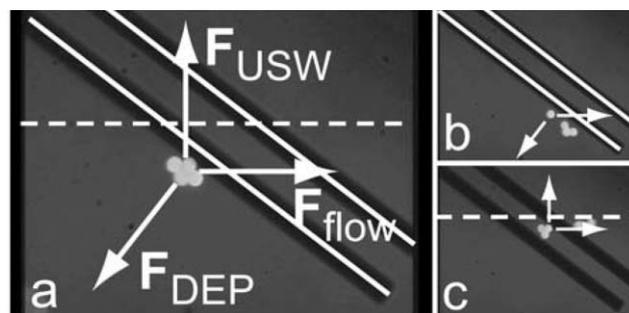
**Fig. 5** The basic principle of combined DEP/USW manipulation, showing the USW, DEP and the flow force components on four trapped particles ( $10 \mu\text{m}$  latex). Each component can be adjusted separately as shown in (b) and (c), resulting in particle selection following trapping. The dotted line marks the USW pressure node and the solid lines mark active electrodes.
