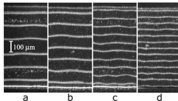
**Fig. 3** Parallel USW alignment in multiple nodes, demonstrated with  $2 \mu\text{m}$  latex. 6 nodes at 6.6 MHz (a), 7 nodes at 7.5 MHz (b), 10 nodes at 10.8 MHz and 13 nodes at 13.4 MHz (d). The experiments are performed without a flow.
