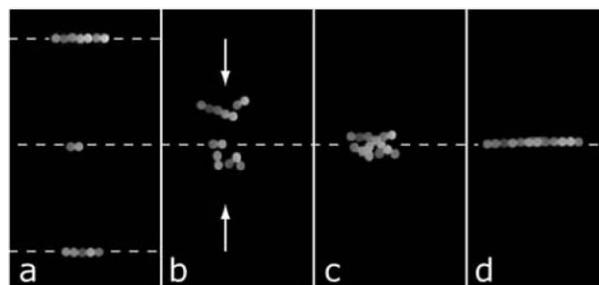
**Fig. 4** Fusion of particle subgroups by ultrasonic frequency shift. Fourteen beads ( $10 \mu\text{m}$  latex) are trapped as line-aggregates in three subsequent nodes at 6.56 MHz (a). When the frequency is changed to 2.12 MHz, the outer nodes are merged with the center node (b–c), resulting in fusion of the three groups into one (d). Dashed lines indicate nodes.
