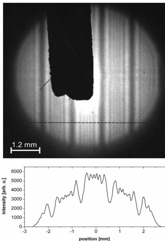
Fig. 3: Interferogram obtained on the CCD detector with an exposure time of 120 s. The dashed line indicates the position of the line plot through the image which is shown below. The large black shadow is the central stop to block the zeroth order<sup>9)</sup>.
