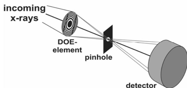
Fig. 2: Experimental arrangement for the testing of the diffractive optical elements.
