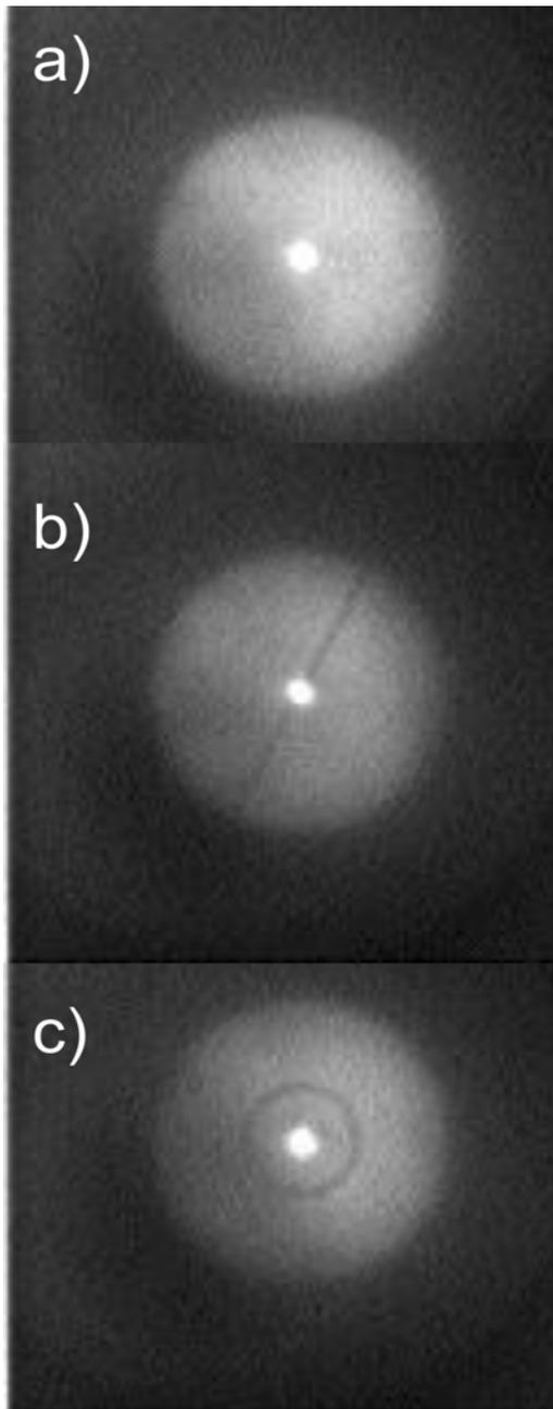
Fig. 4: Interferograms obtained with DOE suited for DIC microscopy: a) normal zone plate +1<sup>st</sup> order cone. b) lateral shear DOE, bias  $\pi$ . c) axial shear DOE, bias  $\pi$ . For details see text.
