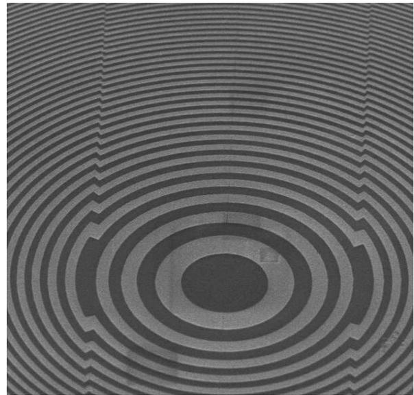
Fig. 1: Electron microscope image of the inner part of a diffractive optical element. Note the phase reversal of the zones in the left and right part of the image.
