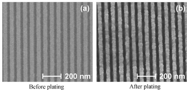
FIG. 7. Scanning electron microscope images of a grating before and after plating with end-point detection. (a) shows 50 nm bright mold lines and 50 nm dark spaces before plating. (b) shows the slightly overplated mold where the nickel is bright and the mold dark.
