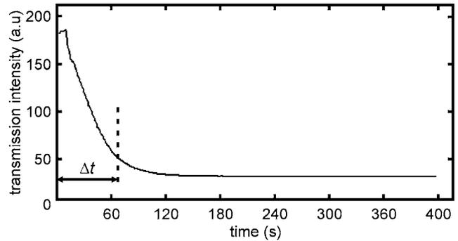
FIG. 4. Light transmission as a function of time during electroplating.
