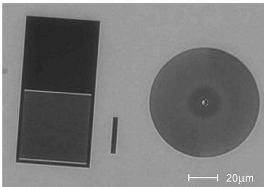
FIG. 3. Transmission light-microscope image recorded during plating of structures on a  $\text{Si}_3\text{N}_4$  membrane. To the right, a  $75 \mu\text{m}$  diameter, 50 nm outermost zone plate. To the left, a test pattern containing a 100 nm period grating (upper) and a large square (lower).
