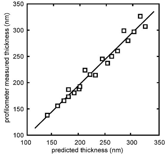
FIG. 5. Correlation between the thickness predicted by the *in situ* transmission-current based method and profilometer measurements.
