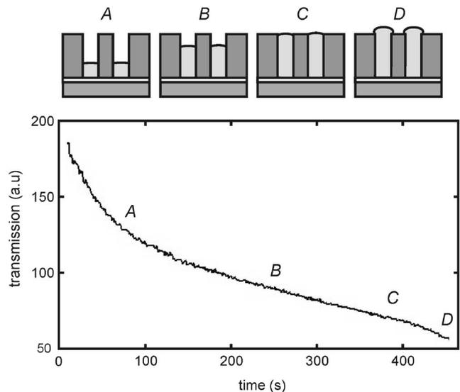
FIG. 6. Experimental recording of the transmission signal through a grating. The different fill ratios are shown schematically on top. Note the drop in intensity at D, which is used for end-point detection.
