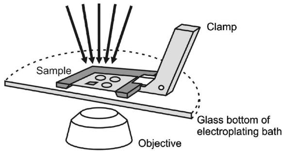
FIG. 2. Experimental arrangement for the optical transmission measurements during the electroplating process.
