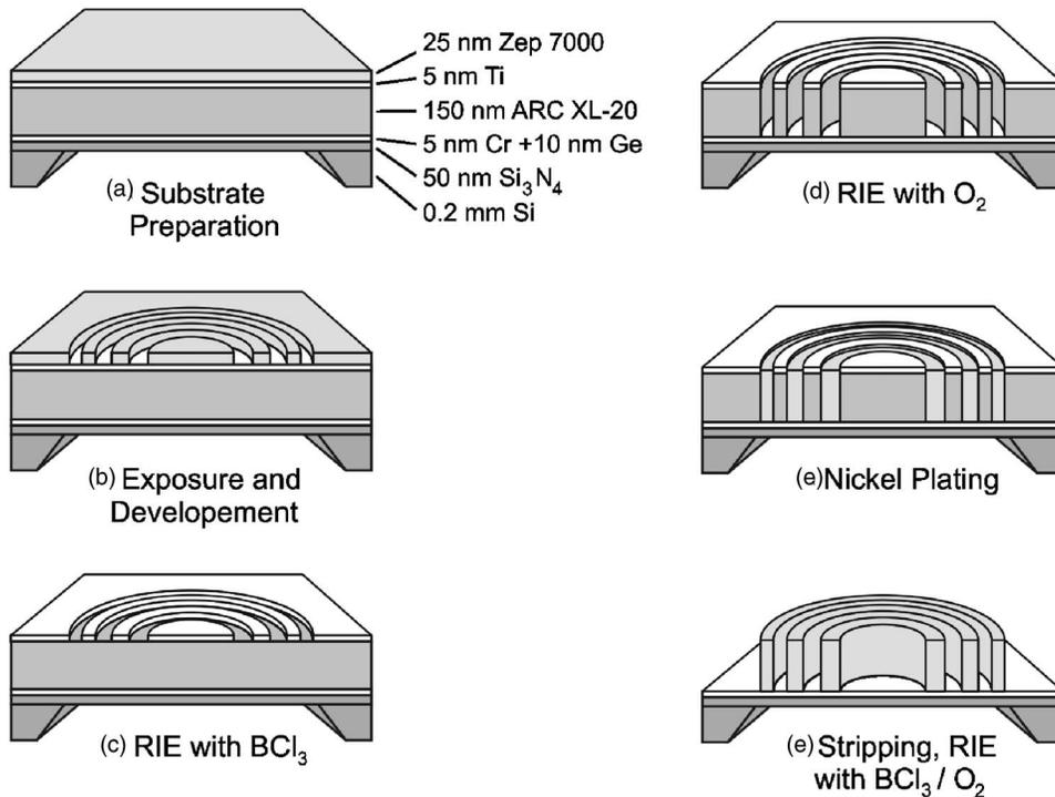
FIG. 1. Process steps for fabrication of high-aspect-ratio zone plates.
