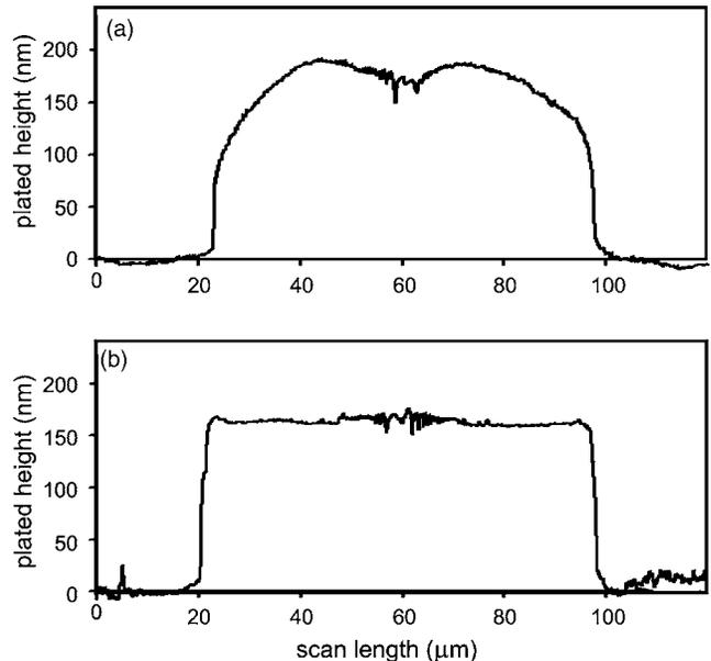
FIG. 4. Height profiles of two zone plates: (a) plated at constant current and (b) plated with optimized pulse reverse plating. The two zone plates are otherwise identical with a 75  $\mu\text{m}$  diameter and an outermost zone width of 50 nm. The oscillations at the middle part of the scans appear because the profilometer tip follows the profile of the relatively large structures at the center of the zone plates.
