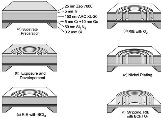
FIG. 2. Trilevel zone plate fabrication process.
