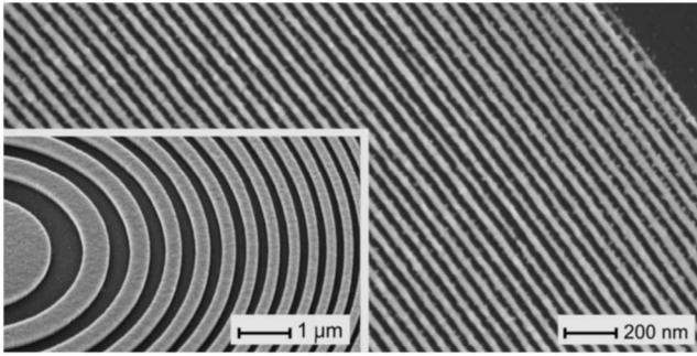
FIG. 1. Outermost and the central part of a nickel zone plate. The outermost zone width is 25 nm and the diameter is 54  $\mu\text{m}$ .
