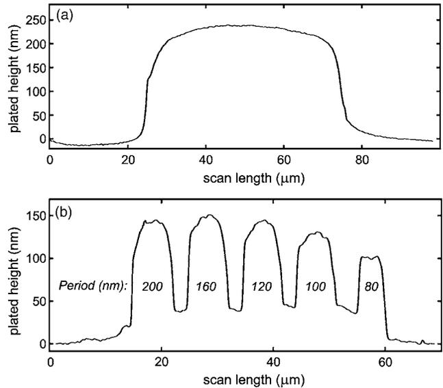
FIG. 3. Profilometer scans showing mass-distribution effects in direct-current plating. (a) Nickel height profile in a  $50 \times 50 \mu\text{m}^2$  unstructured square. (b) Nickel height in gratings of different period.
