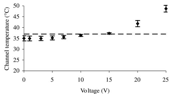
**Figure 4.** The channel temperature measured as a function of an applied transducer voltage ranging from 0 to 25  $V_{pp}$  for an ambient temperature close to 36 °C using the external heating system. The temperature data are averaged from three measurements and the error bars correspond to two standard deviations. The dotted line indicates the physiologically important temperature 37 °C.
