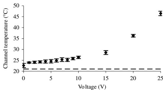
**Figure 3.** The channel temperature measured as a function of an applied transducer voltage ranging from 0 to 25  $V_{pp}$  for an ambient temperature close to 21 °C (indicated by the dotted line). The temperature data are averaged from the three measurements at 2.0 MHz and the error bars correspond to two standard deviations.
