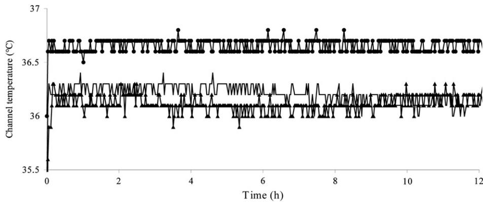
**Figure 2.** The temperature stability during 12 h of particle manipulation is shown in three experiments at a constant transducer voltage of 10  $V_{pp}$  without any flow and with an ambient temperature of 36 °C.
