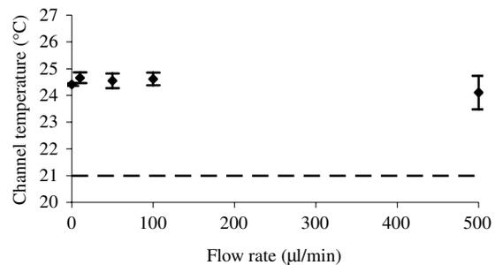
**Figure 5.** The effect on the channel temperature from the flow rate investigated at a transducer voltage of 7 V and with an ambient temperature of 21 °C (indicated by the dotted line). The data are averaged from the three measurements and the error bars correspond to two standard deviations.
