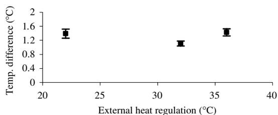
**Figure 6.** The absolute increase in channel temperature evaluated at three different levels of external heating when the transducer is turned on at a constant voltage amplitude of  $10 V_{pp}$ .
