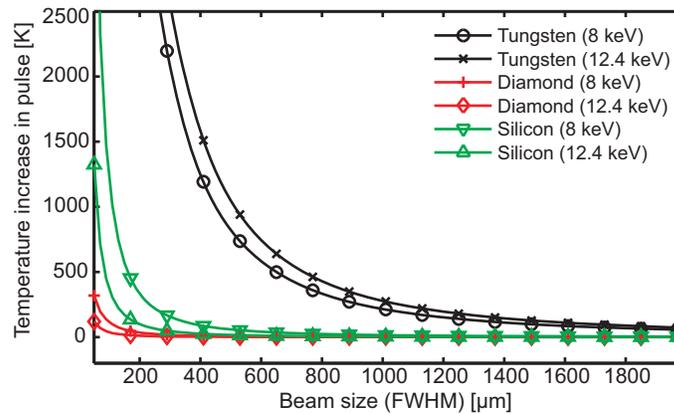
**Figure 3.** Calculated temperature increase in a 2 mJ XFEL pulse for different zone plate materials as a function of beam size. The temperature in the zone plate before the pulse was 300 K.
