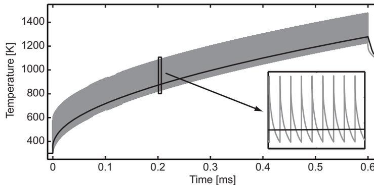
**Figure 5.** Temperature in the center of a 400  $\mu\text{m}$  large and 1  $\mu\text{m}$  thick tungsten zone plate on a diamond substrate during a pulse train of 2700 pulses at the European XFEL. The complete solution including the rapid temperature fluctuations (gray) is compared to the solution obtained from the average intensity (black). The substrate is cooled with a heat transfer coefficient of 0.04  $\text{MW}/\text{m}^2\text{K}$  at a temperature of 300 K.
