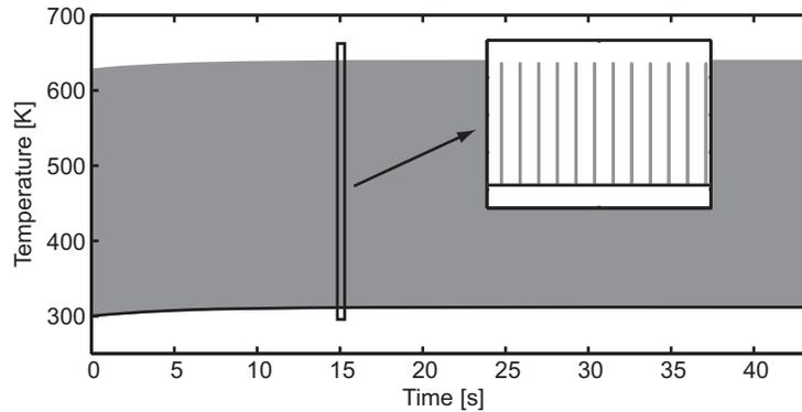
**Figure 4.** Temperature in the center of a 200  $\mu\text{m}$  large and 1  $\mu\text{m}$  thick tungsten zone plate on a diamond substrate in the LCLS beam. The complete solution including the rapid temperature fluctuations (gray) is compared to the solution obtained from the average intensity (black). The substrate is cooled with a heat transfer coefficient of 20  $\text{W}/\text{m}^2\text{K}$  at a temperature of 300 K.
