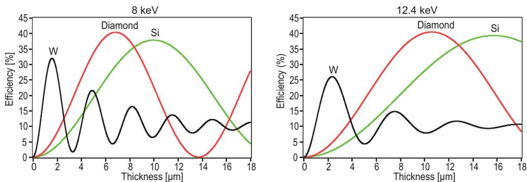
**Figure 1.** Diffraction efficiency of a zone plate in first order as a function of zone thickness at 8 keV and 12.4 keV
