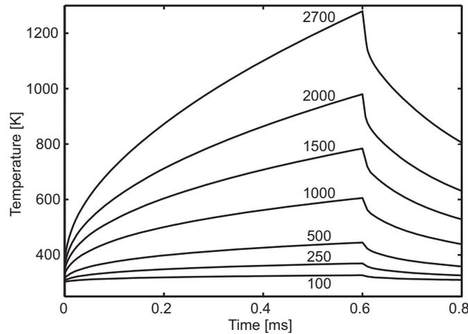
**Figure 7.** Average temperature in the center of a tungsten zone plate on a diamond substrate during a pulse train with varying number of pulses at the European XFEL. Starting temperature was 300 K and  $h = 0.04 \text{ MW/m}^2\text{K}$ .
