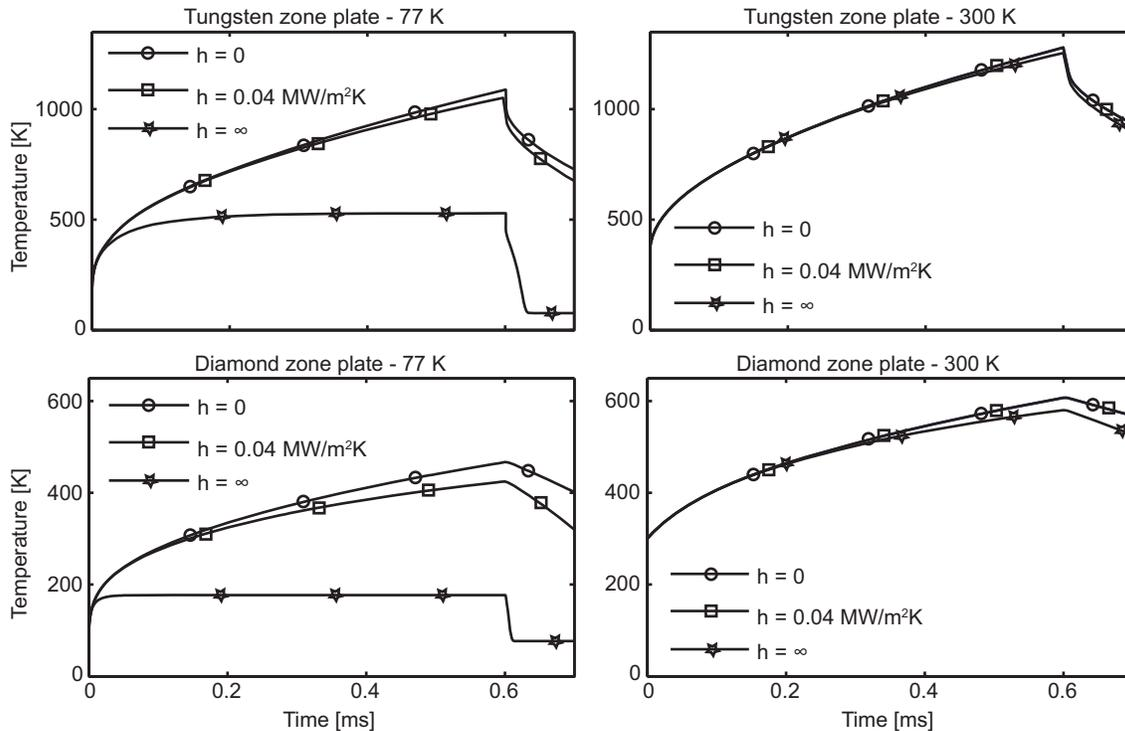
**Figure 6.** Influence of cooling temperature and heat transfer coefficient on the temperature during a pulse train of 2700 pulses at the European XFEL for a tungsten zone plate on a diamond substrate and a pure diamond zone plate. The temperature is the average temperature in the center of the zone plate.
