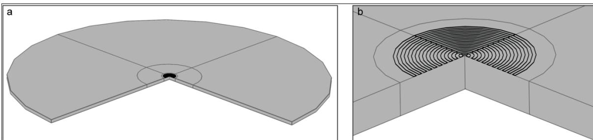
**Figure 2.** (a) 400  $\mu\text{m}$  diameter and 1  $\mu\text{m}$  thick tungsten zone plate on a 10 mm diameter and 100  $\mu\text{m}$  thick diamond substrate (b) Closer look of the same geometry.
