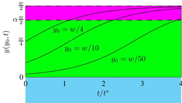
FIG. 2. Transverse particle path  $y(y_0, t)$ , Eq. (3a), as function of normalized time  $t/t^*$ , Eq. (3b). For given fixed parameters, the particle paths (black lines) are plotted for three different starting positions  $y_0$ . The channel is divided into two regions: The interrogation area of relative width  $\alpha$  (green), and the excluded center band of relative width  $1 - \alpha$  (magenta).
