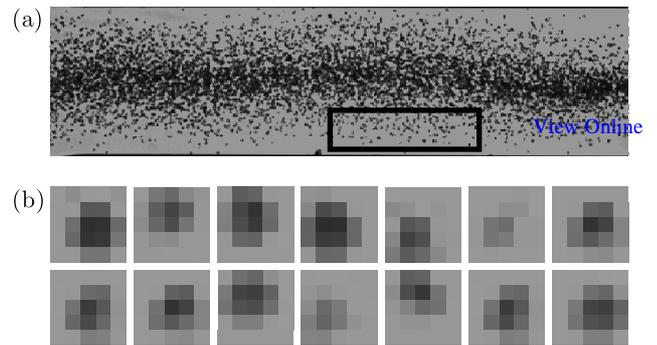
FIG. 5. (a) Gray-scaled experimental image where the microbeads have traversed acoustophoretically half the way towards the center of the microchannel. Inside the black rectangle all isolated particles are identified and their pixel intensities are analyzed within a 5 pixel × 5 pixel square. (b) 5 pixel × 5 pixel square views of 14 of the 41 isolated microbeads in the black rectangle marked in panel (a).
