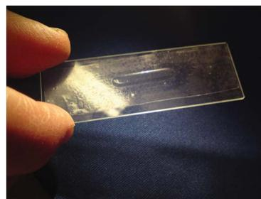
**Fig. 15** Very low cost chambers have been made<sup>52</sup> using the vacuum forming techniques (also used for low cost blister packaging). Driven by pressing, with a clip, against a transducer, as shown in Table 1 **G**.
