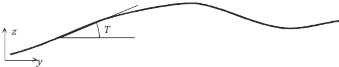
*Figure 8 – A sketch of the bow in the long direction of the SLM. The x-axis is now going into the figure, so the SLM has been turned onto its edge in the sketch [6].*
