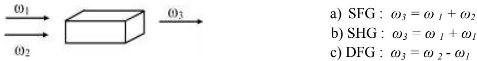
Figure 4.1 Frequency conversion processes in second order nonlinear medium where two input photons are added or subtracted resulting in one photon of higher or lower energy.
