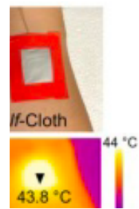
A patch photohermal hybrid material under sunlight.
