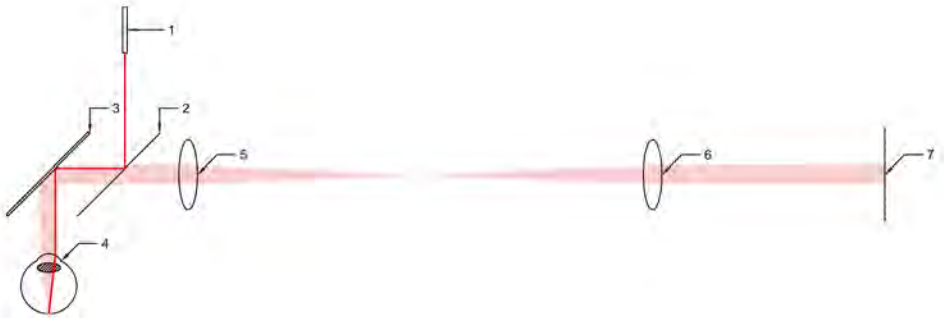
Figure 2.7: A schematic sketch of a one-to-one 4f-Kepler wavefront sensor. Main components are: 1) laser, 2) beam-splitter, 3) hot mirror, 4) eye, 5) first lens (focal length f ), placed f from the exit pupil of the eye, 6) second lens (focal length f , same as first lens) of telescope, placed 2f from the first lens, 7) lenslet array in detector, placed f from the second lens.
