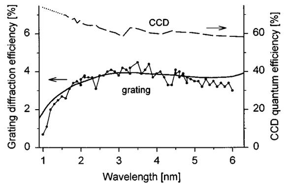
FIG. 5. Calibration curves obtained at BESSY. Symbols/left scale: measured data for the grating diffraction efficiency. Solid line/left scale: calculated values for 110 nm Si and 40 nm Au. Dashed line/right scale: measured CCD quantum efficiency. Dotted: extrapolation to shorter wavelength.
