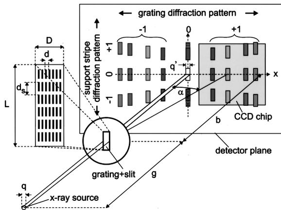
FIG. 1. Working principle of the SGS. The projection shadow of the slit is reproduced by grating diffraction for each wavelength. Aside from the regular diffraction pattern (the spectrum), mixed orders of grating and support stripe diffraction are observed.
