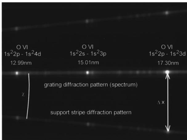
FIG. 10. CCD image taken with SGS in the  $\lambda=12.5\text{--}17.9$  nm range in extreme nonlinear display scaling. The distance  $\Delta x$  between the spectrum and the mixed order  $m=m_s=1$  can be used to determine absolute wavelength.
