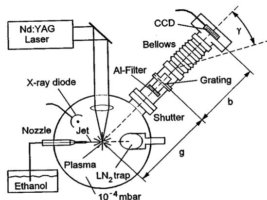
FIG. 6. Experimental arrangement used for the spectral measurements with the SGS.
