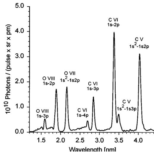
FIG. 8. Absolutely calibrated single shot spectrum (with prepulse).
