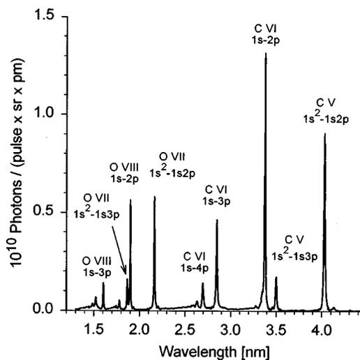
FIG. 7. Absolutely calibrated spectrum of the ethanol jet laser plasma source in the  $\lambda=1.2\text{--}4.4$  nm range.
