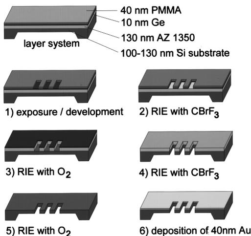
FIG. 2. Nanoprocessing of the freestanding diffraction grating.
