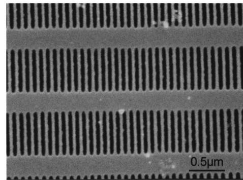
FIG. 3. Electron micrograph of a part of a freestanding diffraction grating with 100 nm  $d$  spacing and 1000 nm period support stripe structure.
