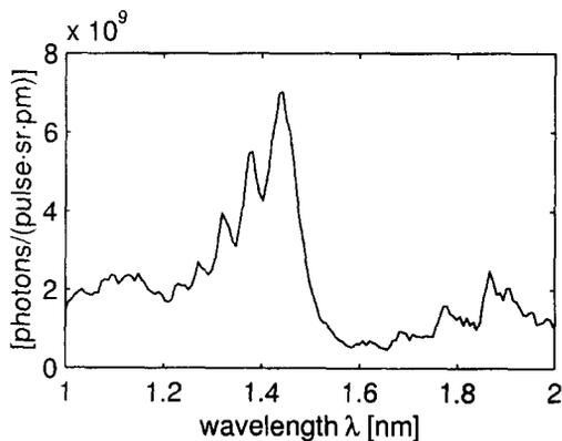
Figure 2. Xe spectrum in the wavelength region suitable for proximity x-ray lithography, showing the average flux of a one-second exposure from a plasma created by 100 Hz of  $\sim 3$  ns long  $\sim 100$  mJ pulses at  $\lambda=532$  nm
