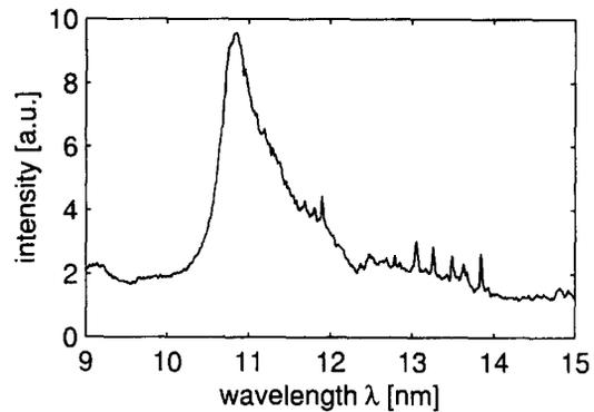
Figure 3. Uncorrected Xe emission spectra in the EUV projection lithography wavelength region.
