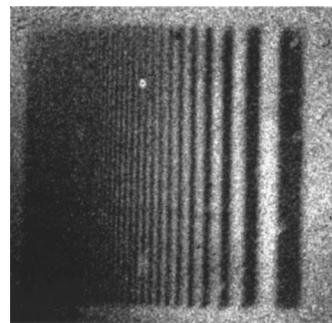
FIG. 3. A 5 min x-ray exposure of a  $10\times 10\ \mu\text{m}^2$  test grating.
