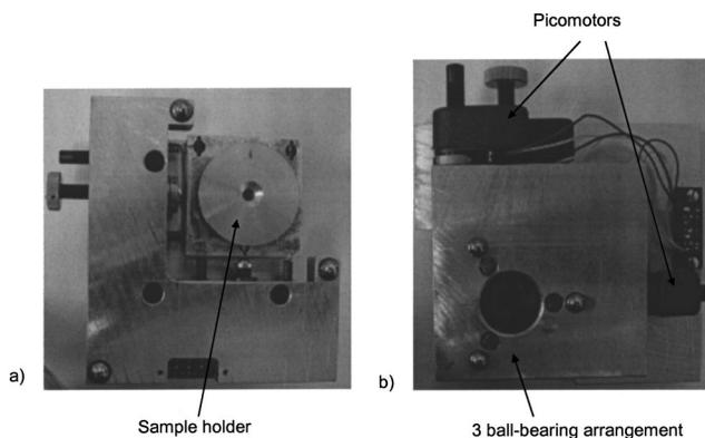
FIG. 2. Photographs of the sample and zone plate holder.
