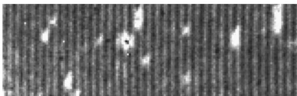
FIG. 4. A 5 min x-ray exposure of a grating with 50 nm structures.
