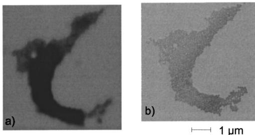
FIG. 5. 80 nm gold spheres on silicon nitride imaged by compact x-ray microscopy (a) and electron microscopy (b).
