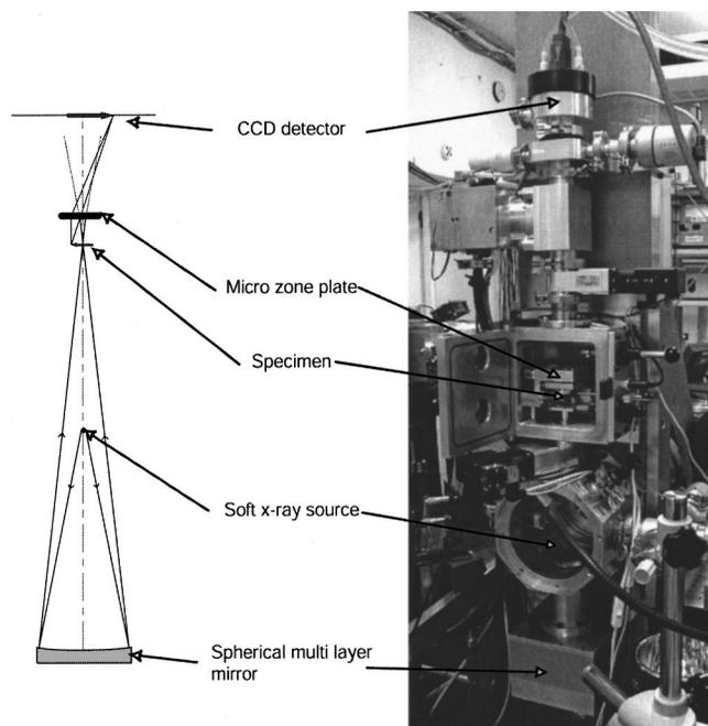
FIG. 1. Experimental arrangement and photograph of the compact x-ray microscope.
