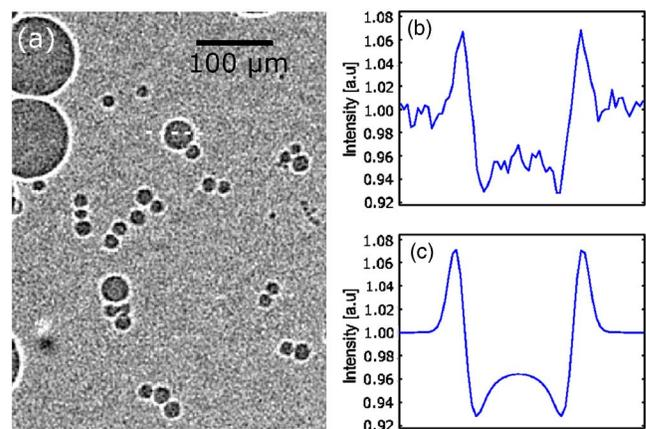
FIG. 3. (a) Phase image of latex beads with different sizes ( $T=180$  s,  $M=5.8$ ,  $r=25$  cm, and  $R=120$  cm). (b) Line scan across a 45 μm diameter bead. (c) Wave-propagation simulation of the imaging of the 45 μm bead.
